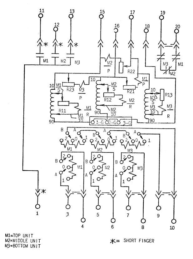
FIG. 1 (0246A3351-0) Internal Connection Diagram For The CEYG51B(-)D Relay
