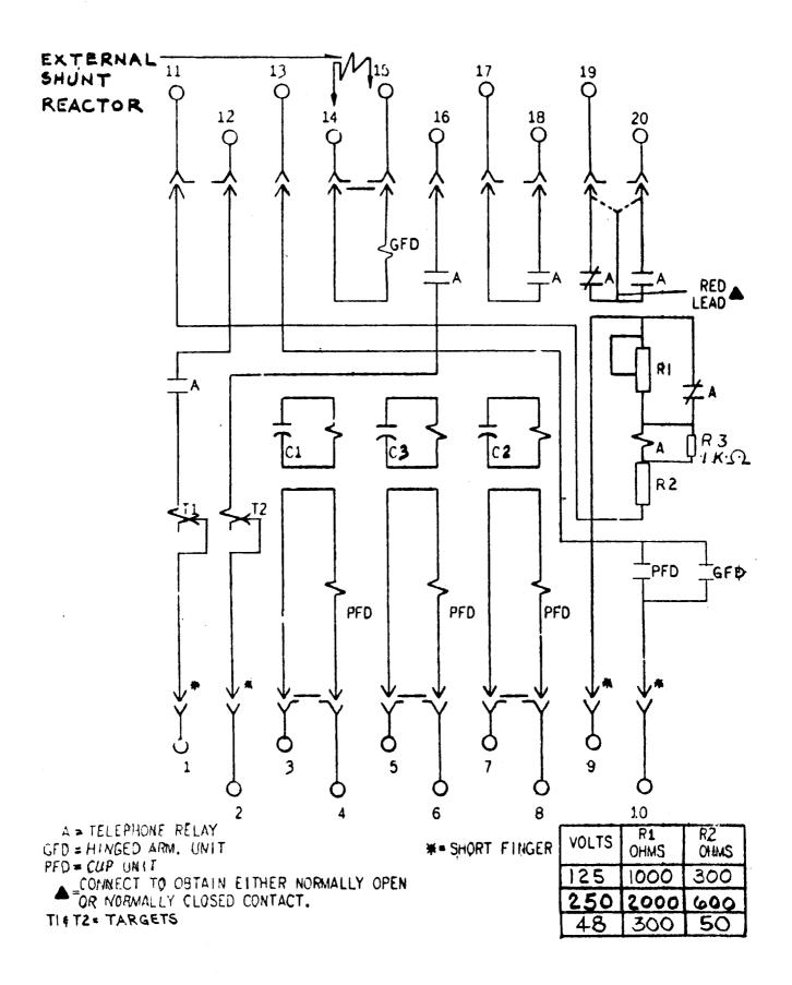
FIG. 1 (0208A2491-4) INTERNAL CONNECTIONS DIAGRAM FOR THE CHC99AD RELAY
