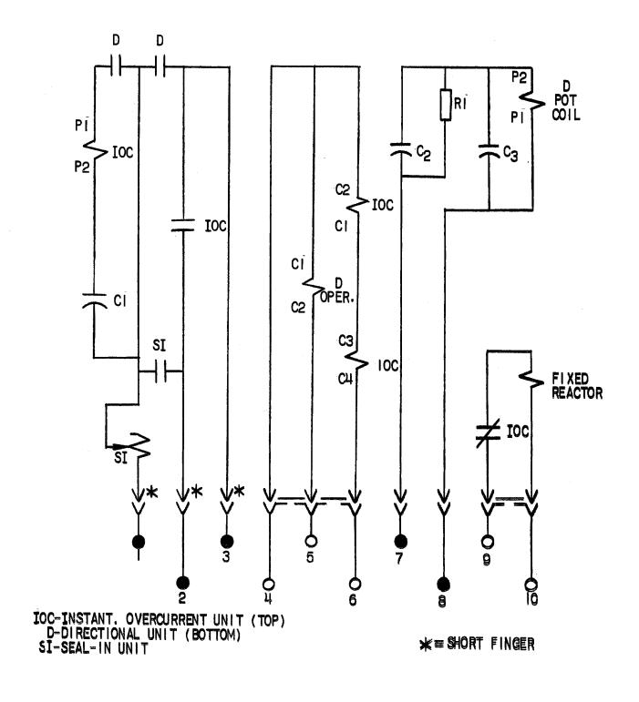
FIG. 1 (0257A8317-0) INTERNAL CONNECTIONS FOR TYPE CJC99AA SPECIAL RELAY
