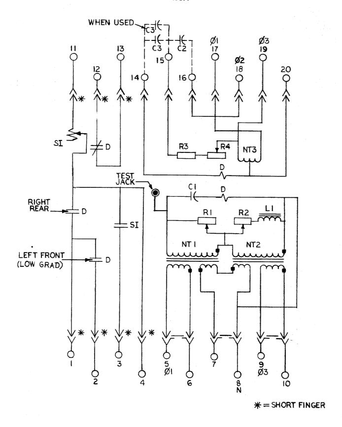
Fig. 1. (0275A2033-1) Internal Connections for 12CNP99AA Relay
