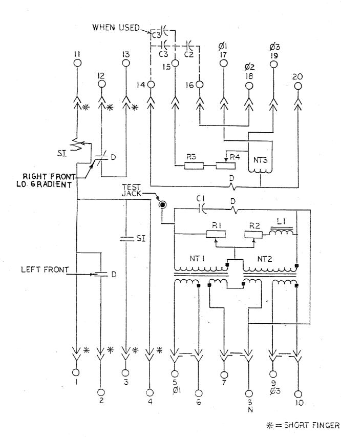
Figure 1 - Internal Connections Diagram (0285A9363-0) 12CNP99AB(-)A RELAY
