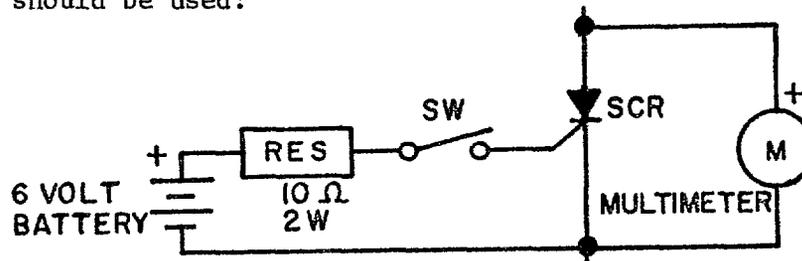
The multi-meter is selected to read ohms on the 1K scale, and is connected to read the forward resistance of the SCR. When switch SW is closed, the forward resistance of a good SCR will change from a high value (100K to infinity) to a low value (1 to 10K). When the switch is opened, a good SCR will revert to its high forward resist-
