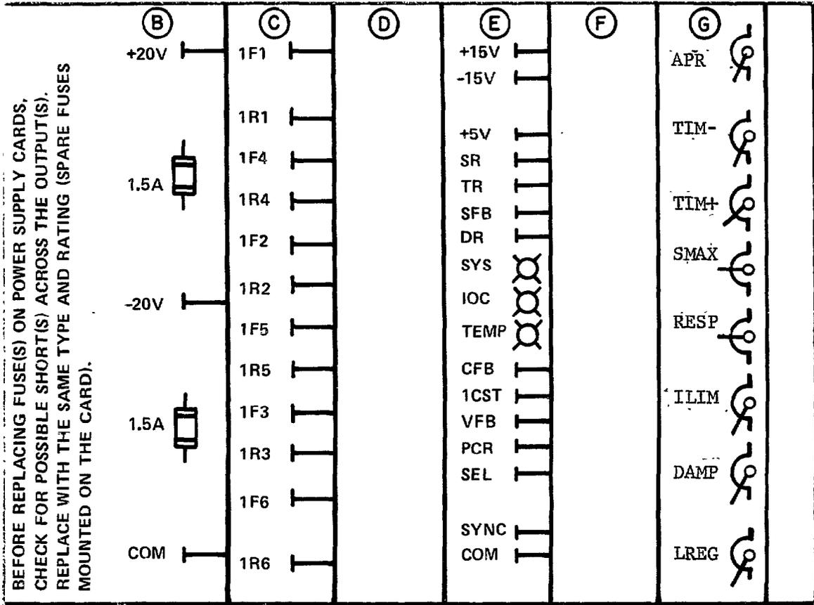
BEFORE REPLACING FUSE(S) ON POWER SUPPLY CARDS, CHECK FOR POSSIBLE SHORT(S) ACROSS THE OUTPUT(S). REPLACE WITH THE SAME TYPE AND RATING (SPARE FUSES MOUNTED ON THE CARD).
