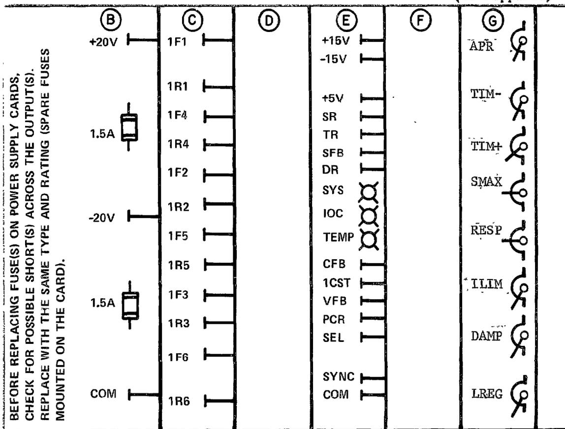
BEFORE REPLACING FUSE(S) ON POWER SUPPLY CARDS, CHECK FOR POSSIBLE SHORT(S) ACROSS THE OUTPUT(S). REPLACE WITH THE SAME TYPE AND RATING (SPARE FUSES MOUNTED ON THE CARD).
