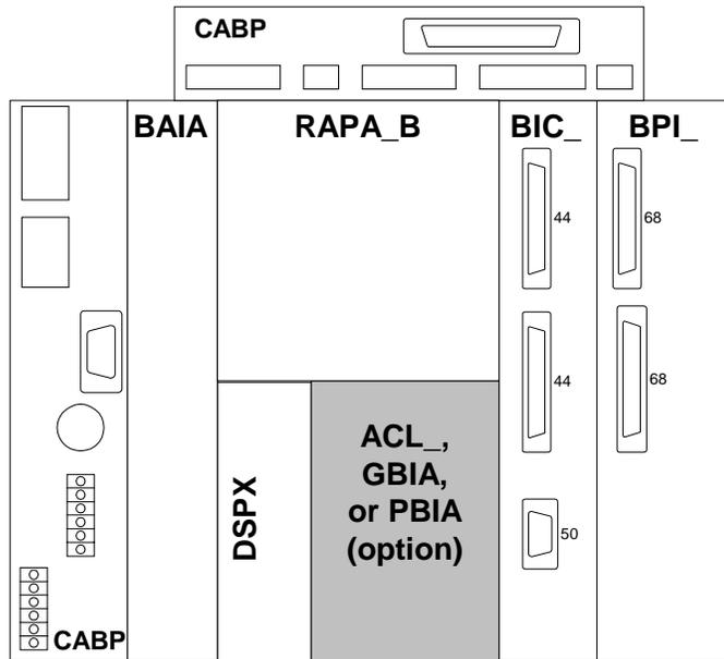
Figure 8. GBIA Module Location in the Board Rack
