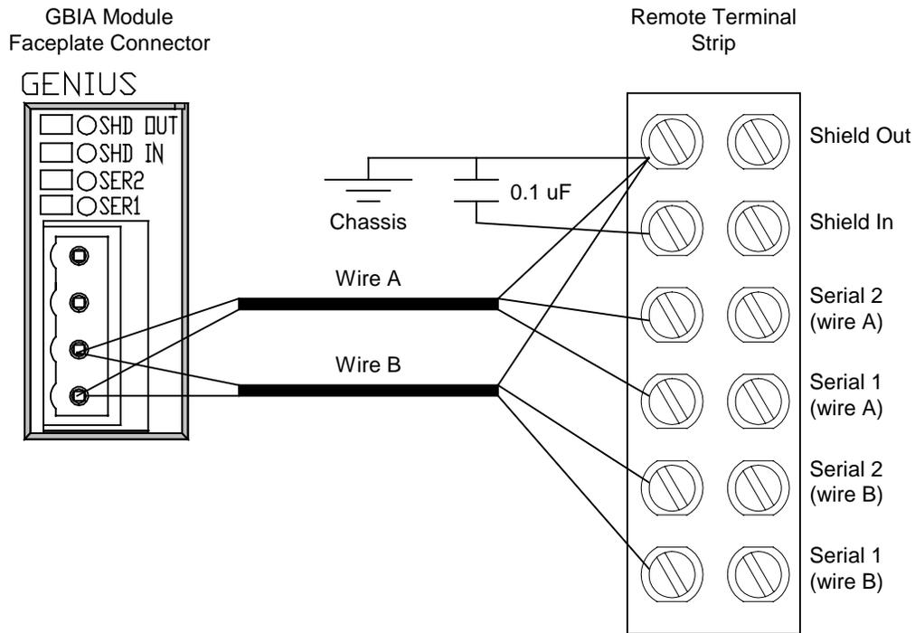
Figure 4. Remote Terminal Strip Genius Bus Connection
