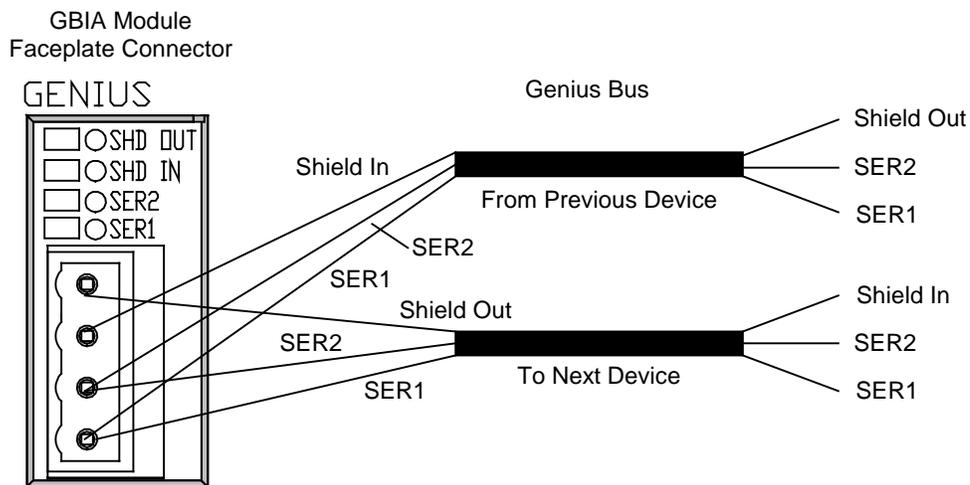
Figure 3. Direct Connection to Genius Bus
