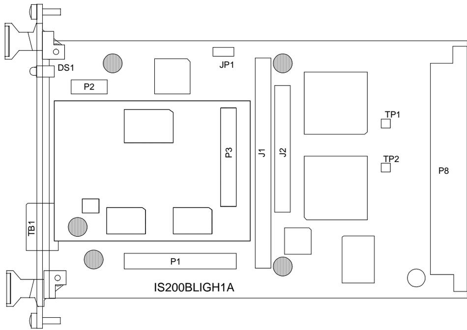
Figure 7. GBIA Module (BLIG Board) Layout Diagram
