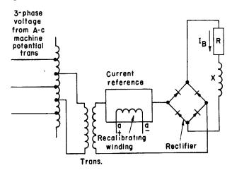
Fig. 3. Elementary diagram of the reference circuit
