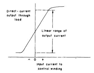
Fig. 8. Characteristic curve of a magnetic amplifier
