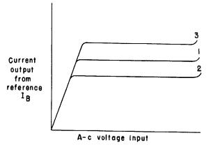
Fig. 4. Curves of reference-circuit output current vs. three-phase potential-transformer voltage showing effect of recalibrating winding a-a
