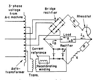
Fig. 5. Elementary diagram of the comparison circuit which is composed of the averaging circuit (Fig. 1) and the reference circuit (Fig. 3)
