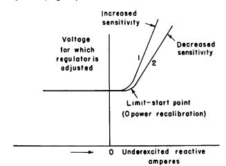
Fig. 12. Curves of underexcited reactive amperes vs. regulator voltage, showing effect of limitsensitivity adjustment
