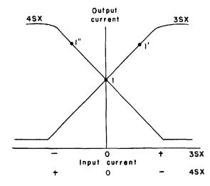
Fig. 11. Characteristic curves of second-stage magnetic amplifier
