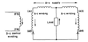
Fig. 7. Elementary diagram showing windings of a magnetic amplifier
