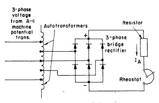
Fig. 1. Elementary diagram of the averaging circuit
