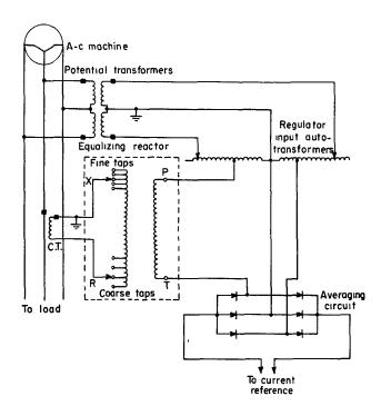
Fig. 14. Equalizing-reactor connections
