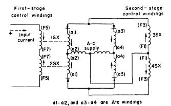
Fig. 9. Elementary diagram of the first stage of the balanced magnetic amplifier
