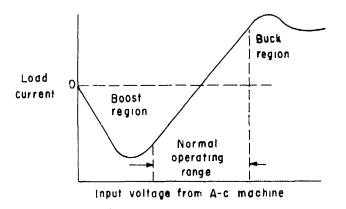
Fig. 6. Curve of comparison circuit output current vs. input voltage from the a-c machine
