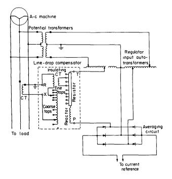
Fig. 15. Line-drop compensator connections
