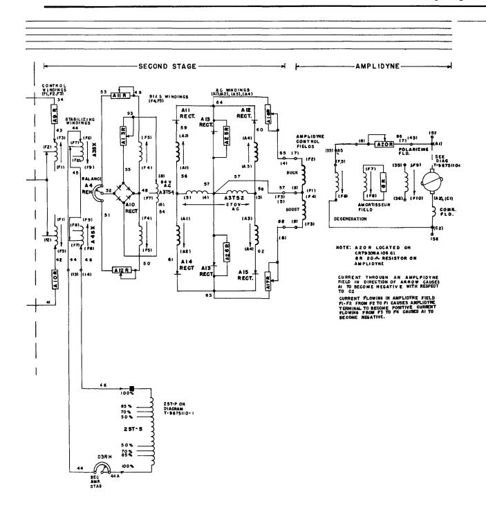
Fig. 17 Typical elementary diagram of the voltageregulator circuit (T-9675110-2)
