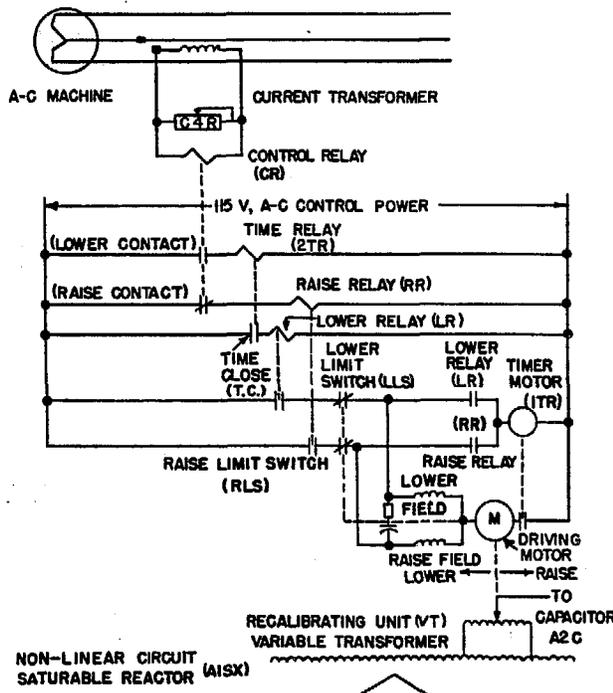
Fig. 15. Maximum excitation limit circuit
