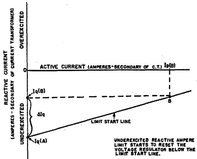
Fig. 20. Typical limit start characteristics.
