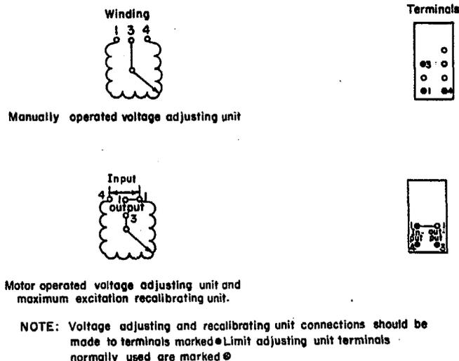
**Fig. 16. Variable transformer internal connections**
