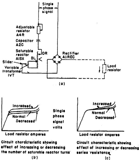
Fig. 2. Nonlinear circuit and its signal voltage—load current characteristic
