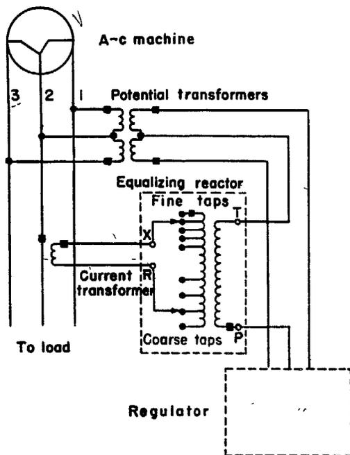
Fig. 13. Equalizing-reactor connections
