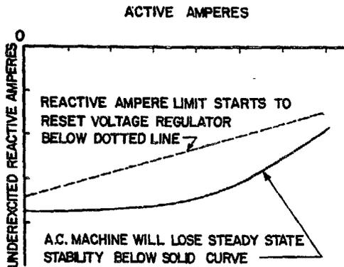
Fig. 4. Typical a-c machine pull-out and reactive-ampere limit-start characteristics
