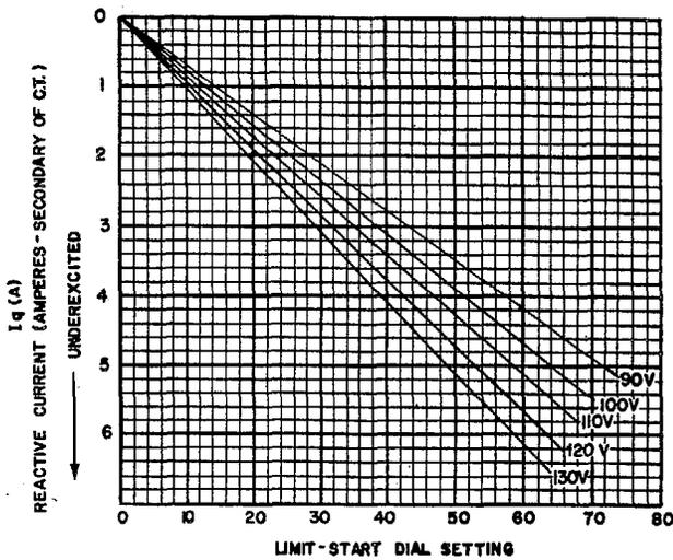
Fig. 18. Calibration curves for reactive-ampere limit start dial
