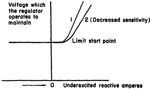
Fig. 9. Reactive-ampere limit sensitivity adjustment characteristic
