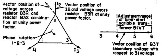
Fig. 5. Vector positions of input quantities of reactive-ampere sensitive circuit
