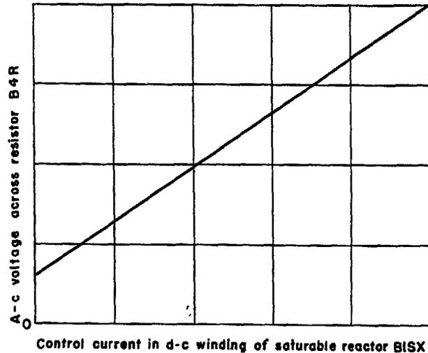
Fig. 10. Characteristic of voltage-resetting circuit
