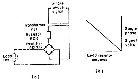
Fig. 1. Linear circuit and its signal voltage—load current characteristic
