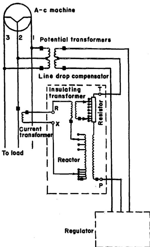
Fig. 14. Line-drop compensator connections
