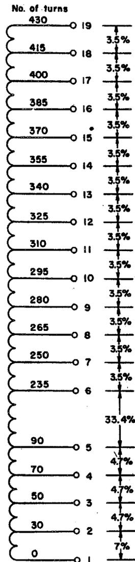
Numbers indicate corresponding winding taps and terminal numbers. Percentage figures refer to percentage of total winding between respective taps.
