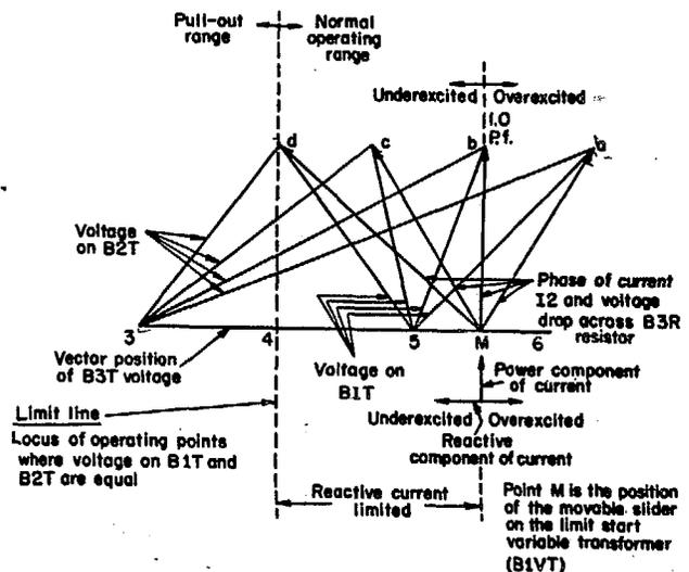
Fig. 6. Vector diagram for reactive-ampere sensitive circuit without power recalibration reactance in circuit
