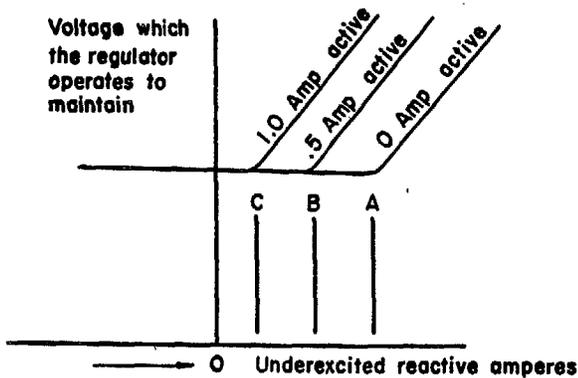
Fig. 7. Reactive-ampere limit power recalibration characteristic
