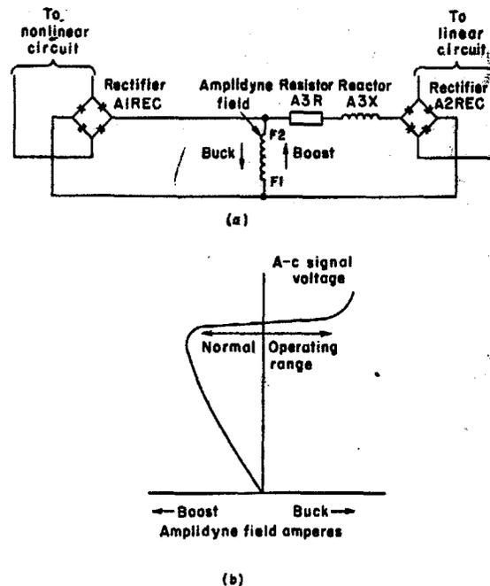
Fig. 3. Comparison circuit and its signal voltage—amplidyne field current characteristic
