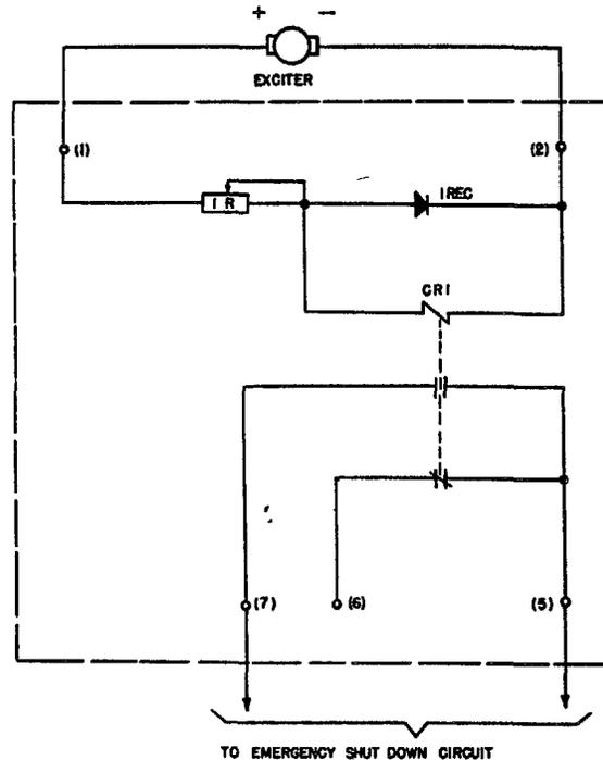
Fig. 17. Exciter voltage relay panel
