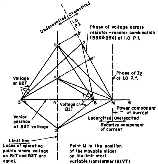
Fig. 8. Vector diagram for reactive-ampere sensitive circuit with some power recalibration reactance in circuit
