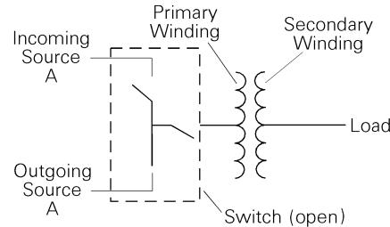
Figure 21. Schematic of the loop-radial switch.
