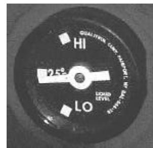
Figure 2. Liquid-level gage accessory.
