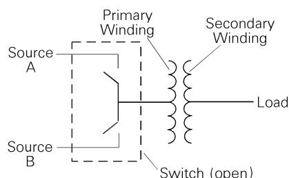
Figure 22. Schematic of the interlocked alternate-source switch.
