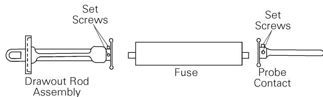
Figure 10. Loadbreak dry-well fuse replacement.
