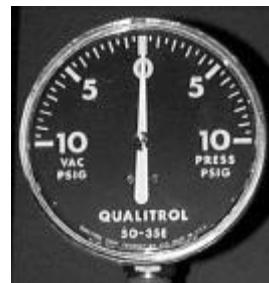
Figure 3. Pressure vacuum gage accessory.
