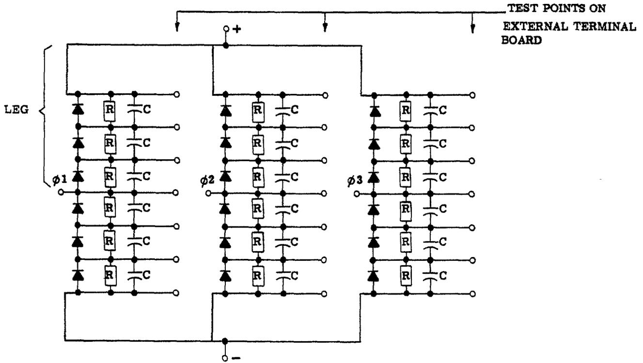
Figure 5. Rectifier Electrical Connections
