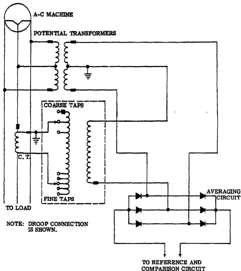
Figure 8. Reactive Current Compensator Connections
