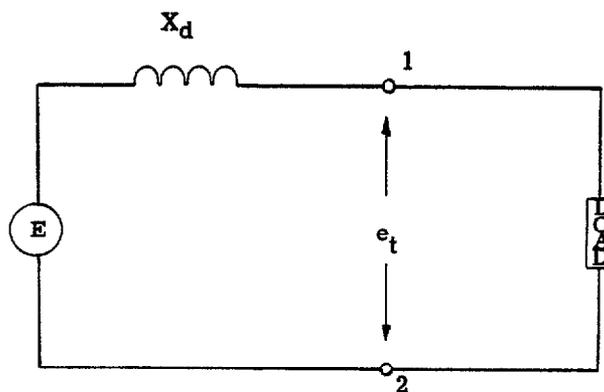
Figure 4. Simplified Generator Equivalent Circuit
