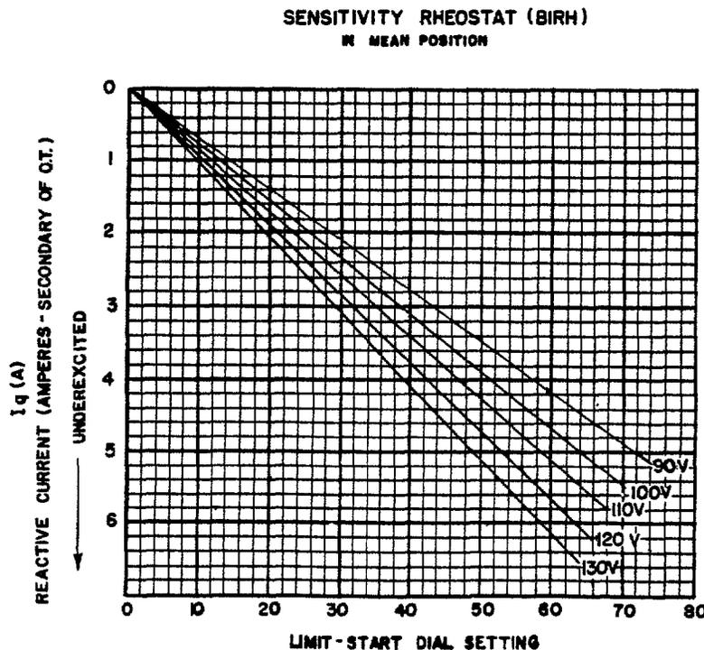
Figure 10. Calibration Curves For Reactive Ampere Limit Start Dial
