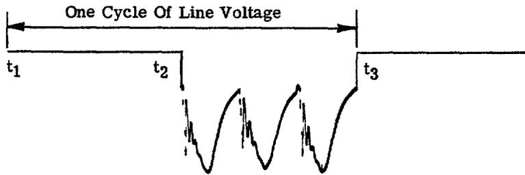
Figure 6. Voltage Across Normal Diode
