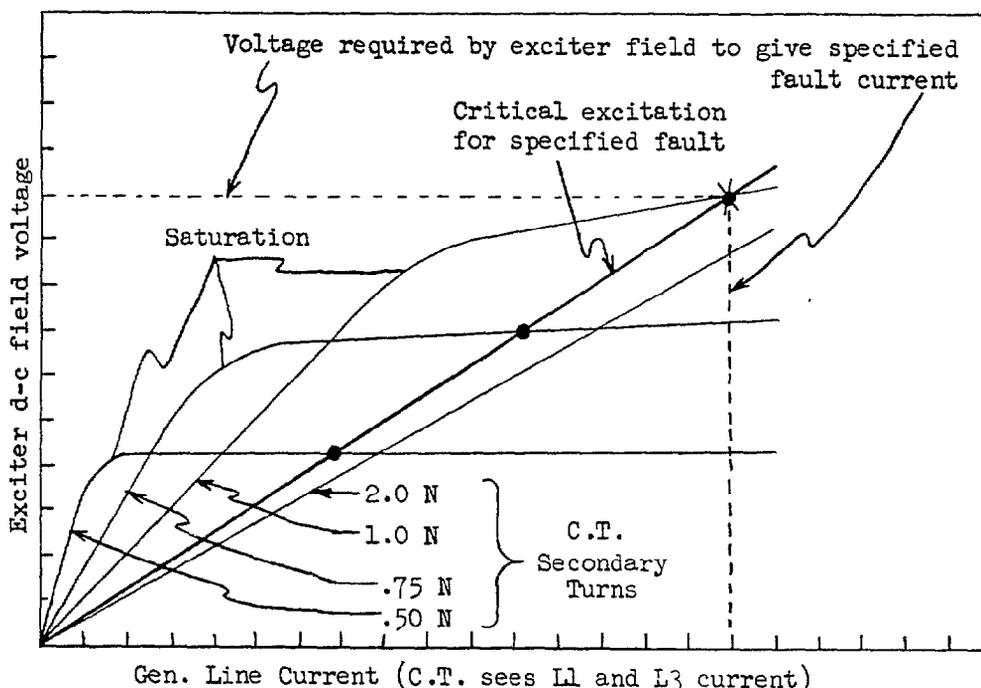
Figure 5. Action of Saturating C. T. on Faults
