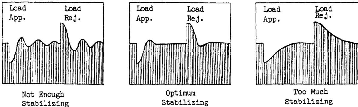
Figure 1. Typical Oscillograms Looking at an Amplified Portion of Generator A-C Voltage
