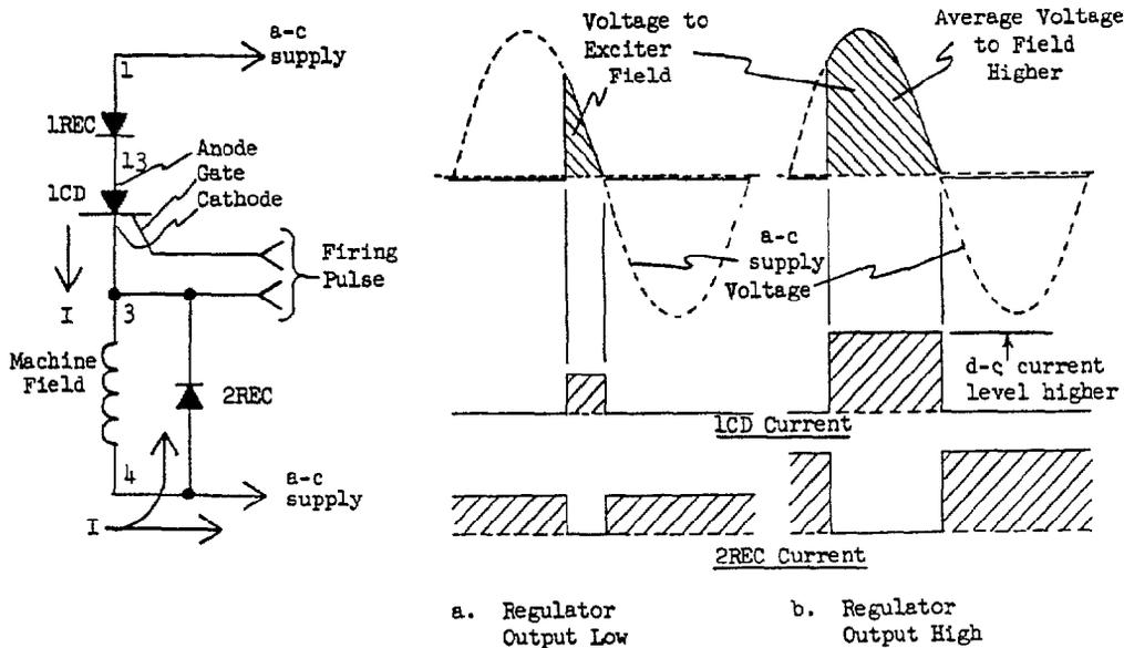
Figure 2. Phase Controlled Output of SCR (1CD)
