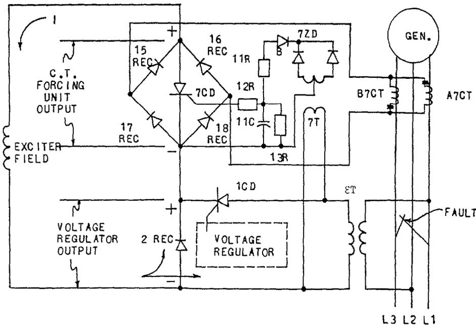
Figure 4. C. T. Forcing Unit Operation
