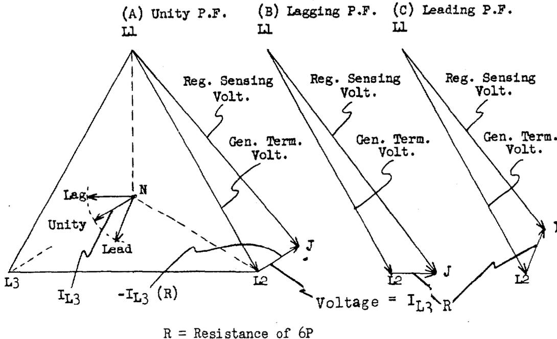
Figure 6. Operation of Paralleling (Droop) Circuit
