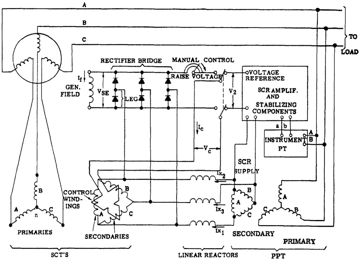
Figure 1. Simplified Static Exciter-Regulator System
