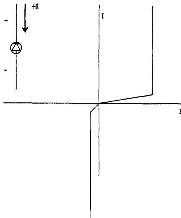
Figure 6. Current-voltage Characteristics of a Zener Diode
