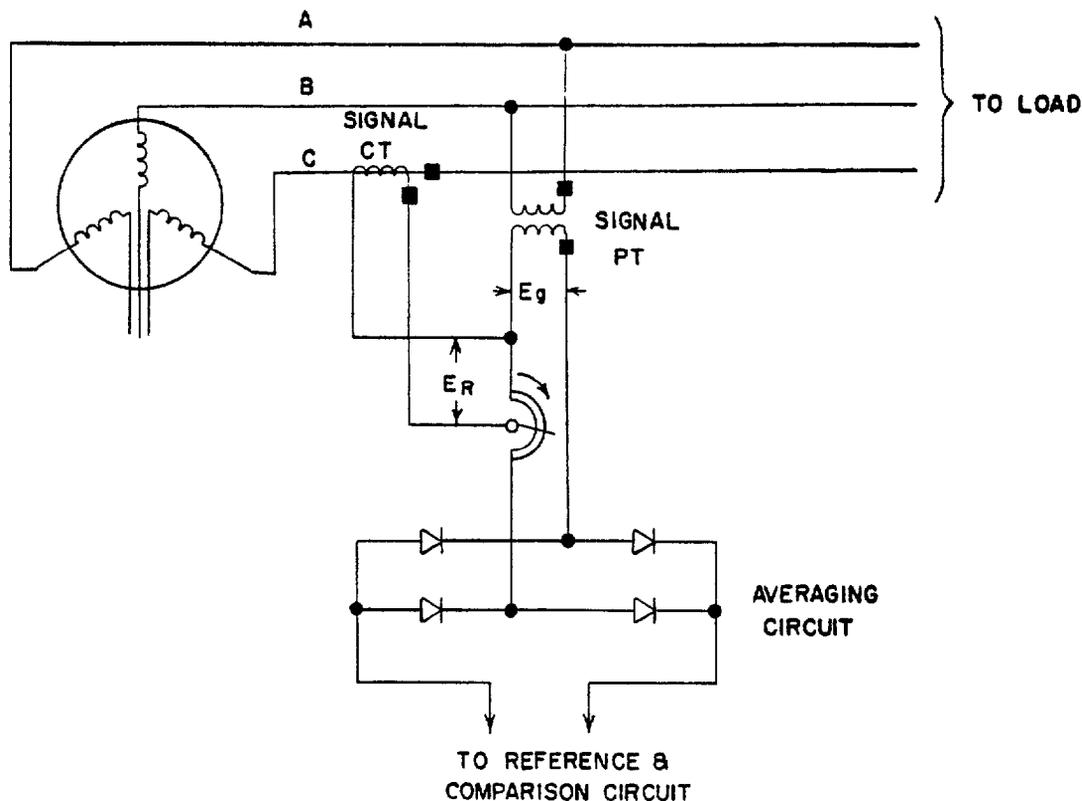
Figure 9. Reactive Current Compensator
