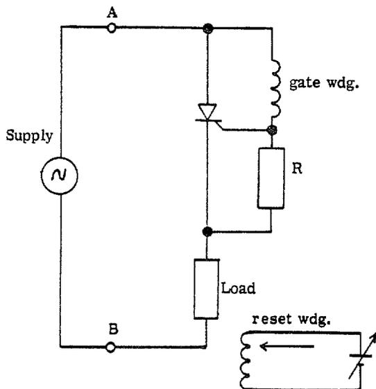
Figure 7. Simplified Version of SCR Circuit
