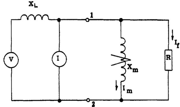
Figure 2. Equivalent Circuit of Saturable C. T. Type Static Exciter
