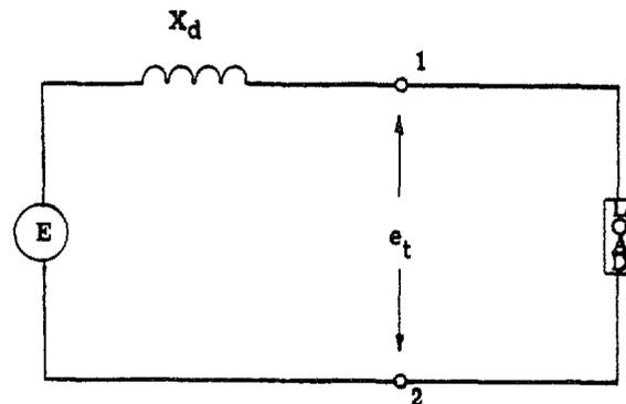
Figure 4. Simplified AC machine Equivalent Circuit
