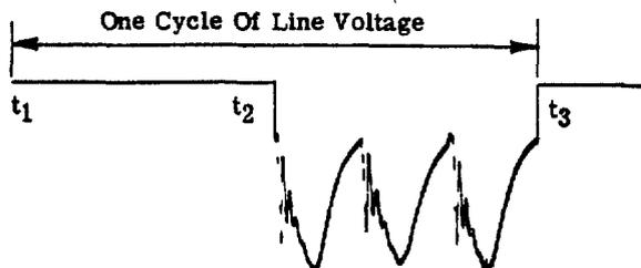
Figure 5. Wave-form Across One Diode When Operating Properly
