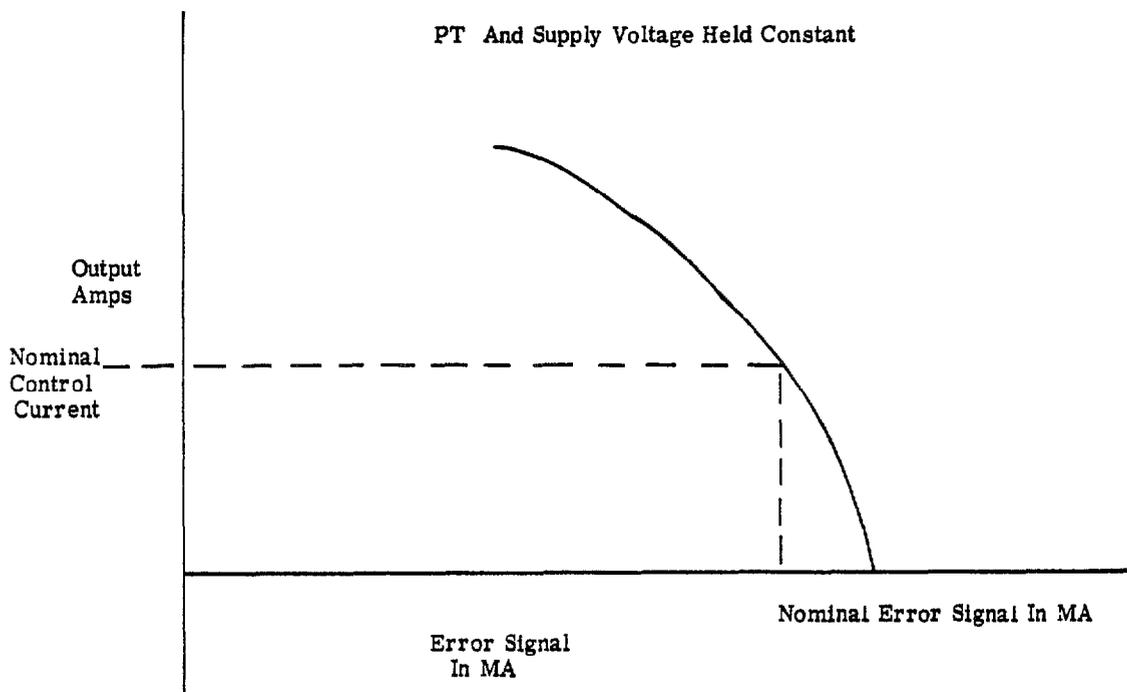
Figure (8b) Comparison Circuit Output
