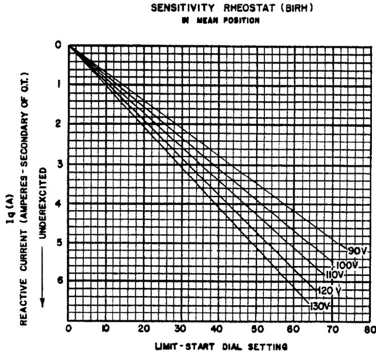
Figure 10. Calibration Curves For Reactive Ampere Limit Start Dial
