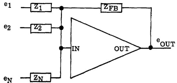
$$e_{OUT} = -e_1 \frac{Z_{FB}}{Z_1} - e_2 \frac{Z_{FB}}{Z_2} \dots - e_N \frac{Z_{FB}}{Z_N}$$
