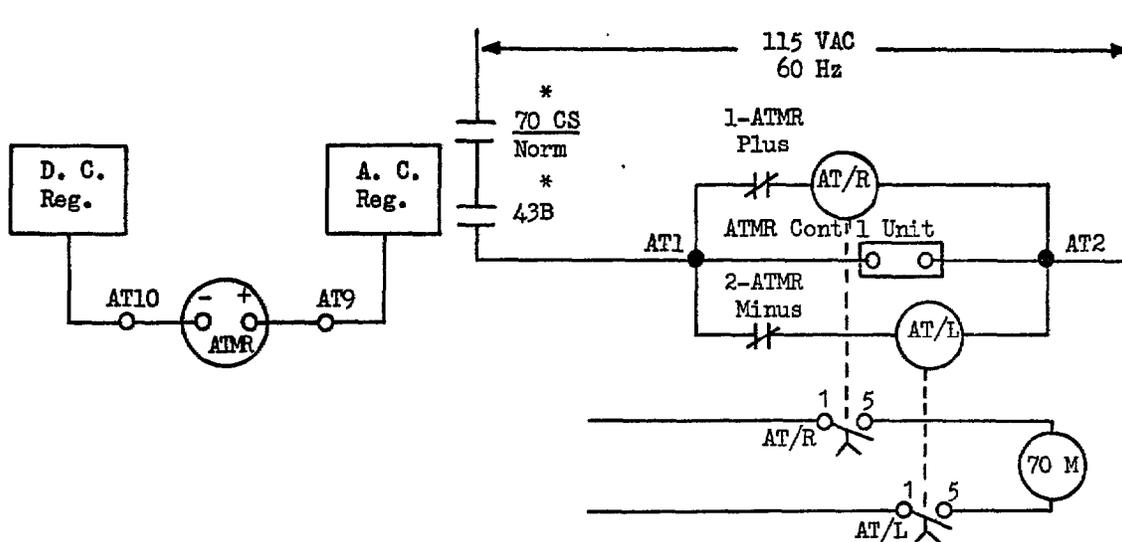
Figure 1 - Automatic Tracking Panel Typical Hook-Up
