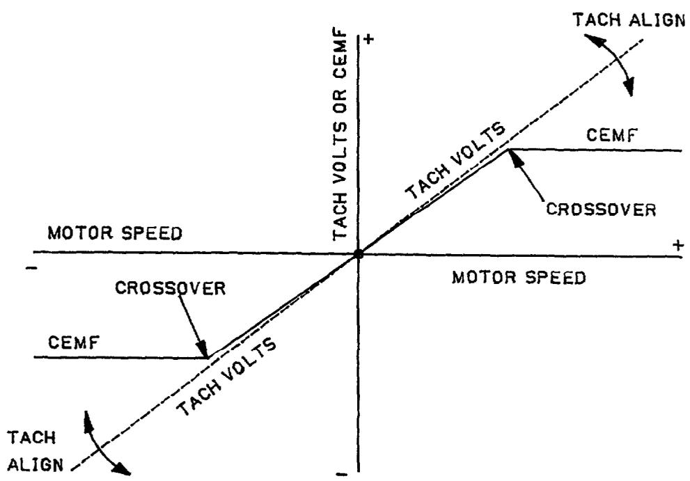
FIGURE 4. RELATIONSHIPS BETWEEN CEMF, TACHOMETER VOLTS, MOTOR SPEED CROSS AND ALIGN ADJUSTMENTS
