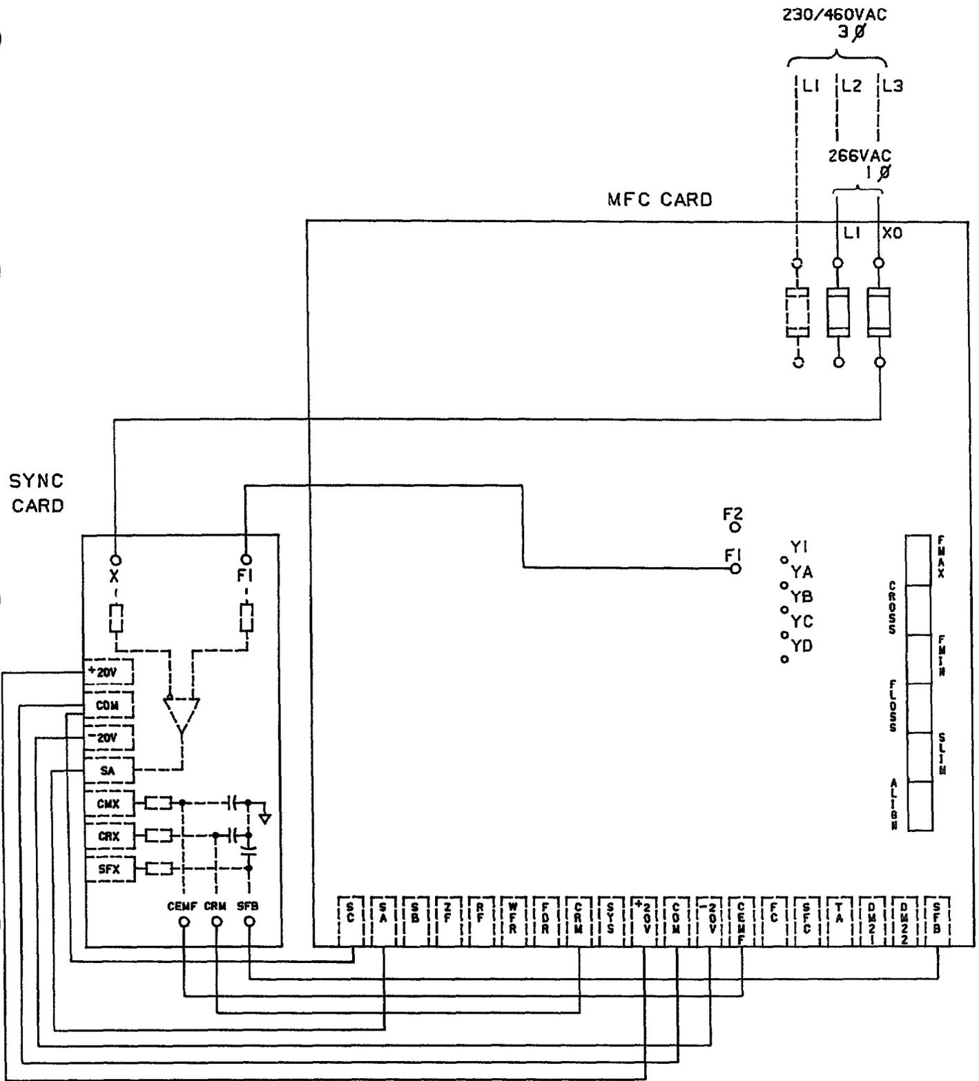
FIGURE I. ASSEMBLY CONNECTION DIAGRAM
