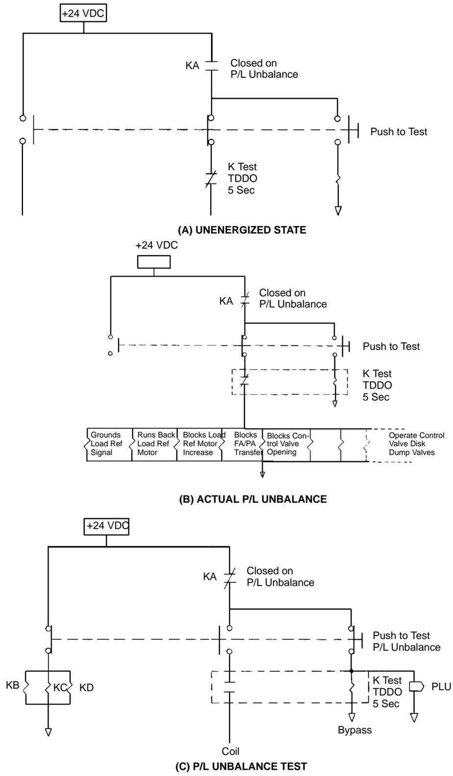
Figure 2. Power / Load Unbalance Logic
