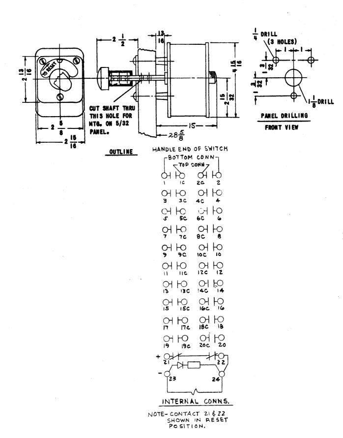
FIG. 1 (0208A8141-1 Sh.2) Outline and Panel Drilling Dimensions and Internal Connections Diagram for the 0208A8141 HEA Special Relay.
