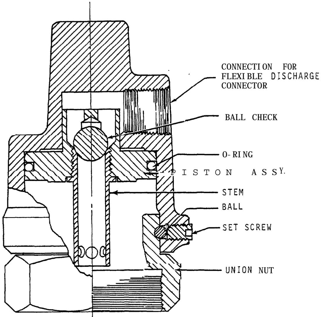
Figure 5. Pneumatic Operated Heads.
