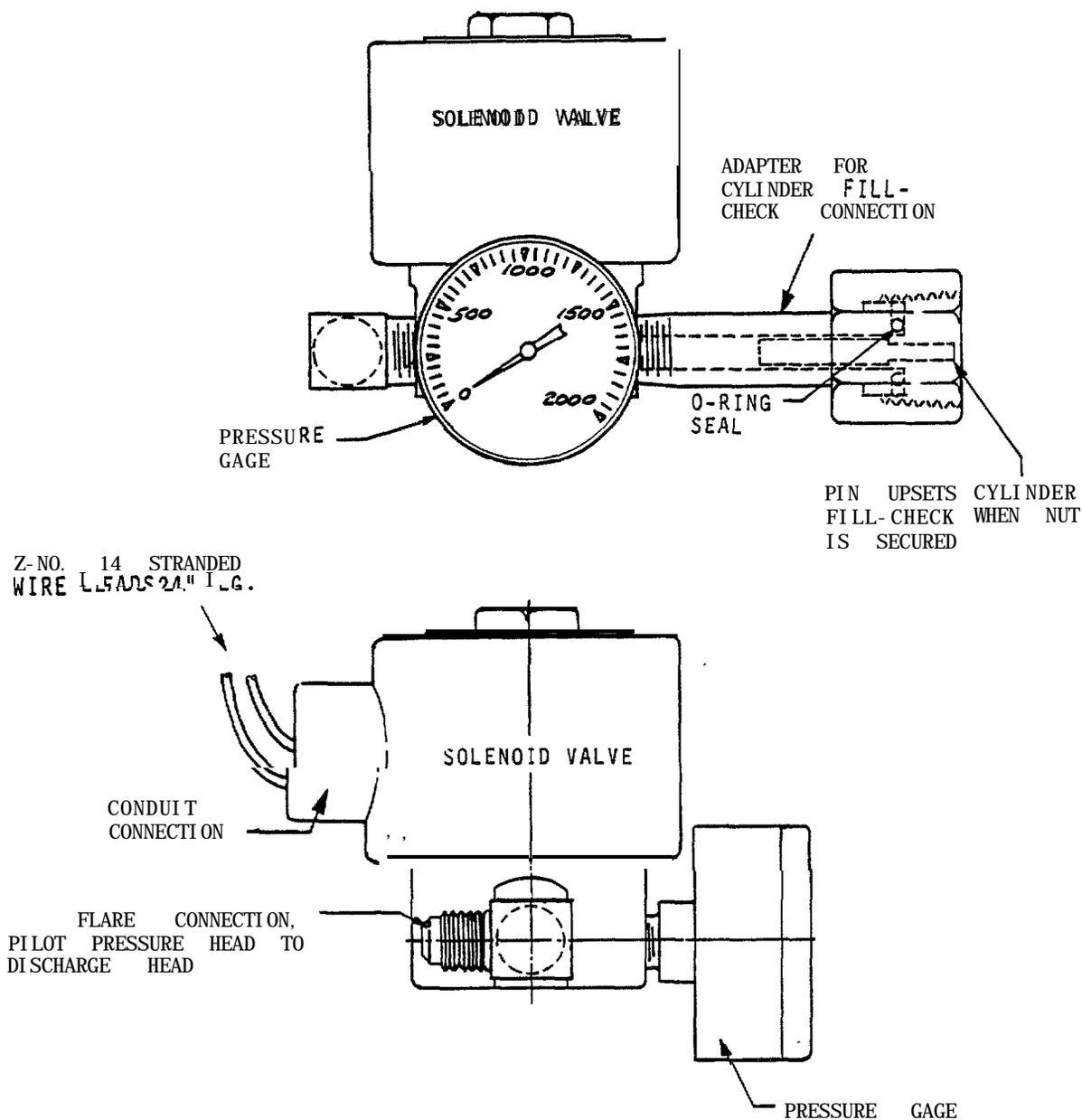
Figure 1. Solenoid Pilot Valves 45CR-1 and 45CR-2.
