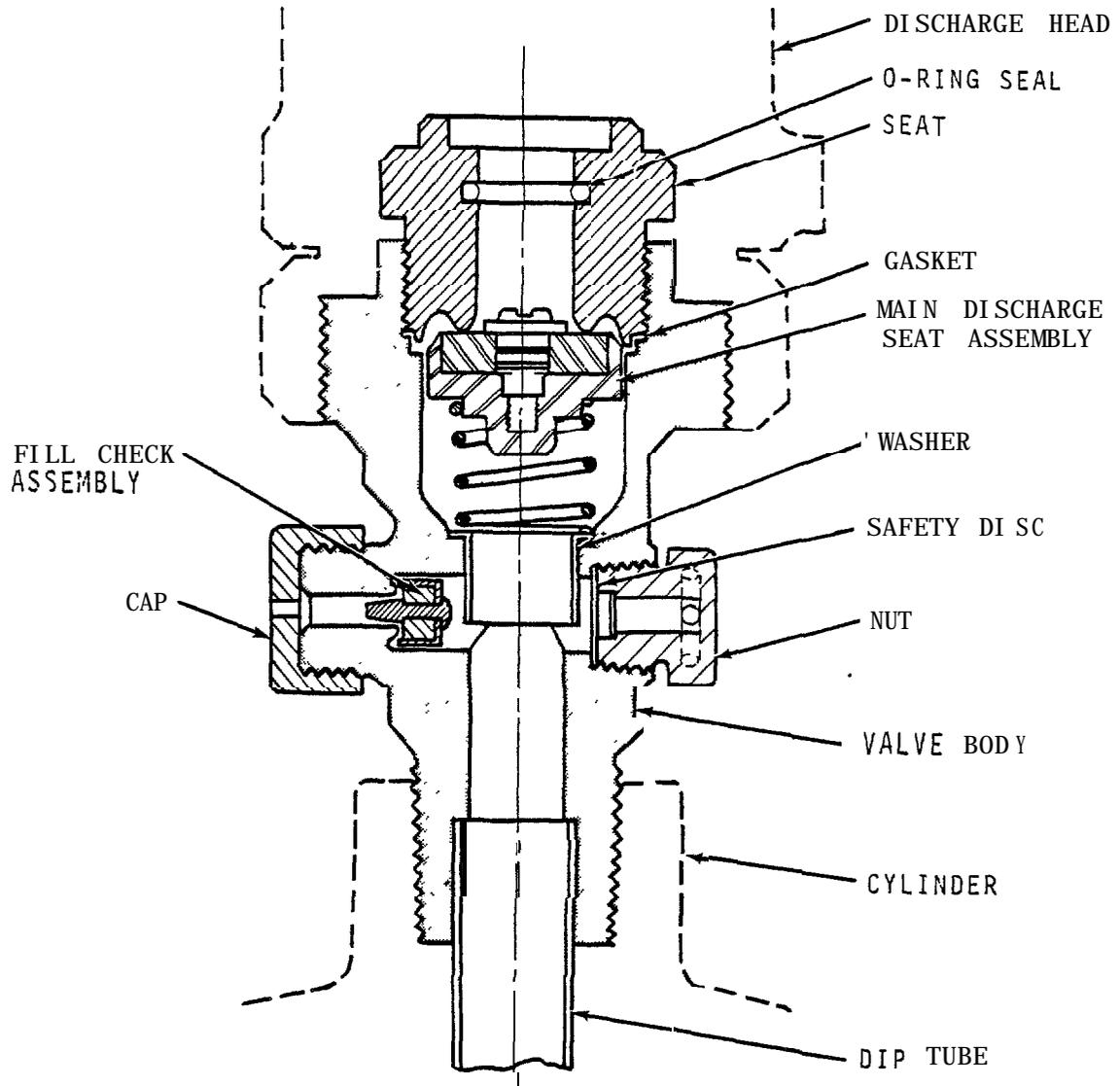
Figure 7. Cylinder Valve and Dip Tube.
