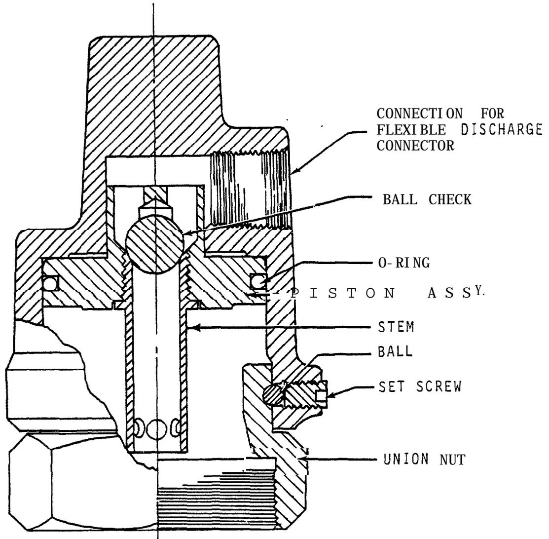
Figure 5. Pneumatic Operated Heads.
