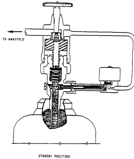
Figure 24. Pilot Cylinder Discharge Heads.
