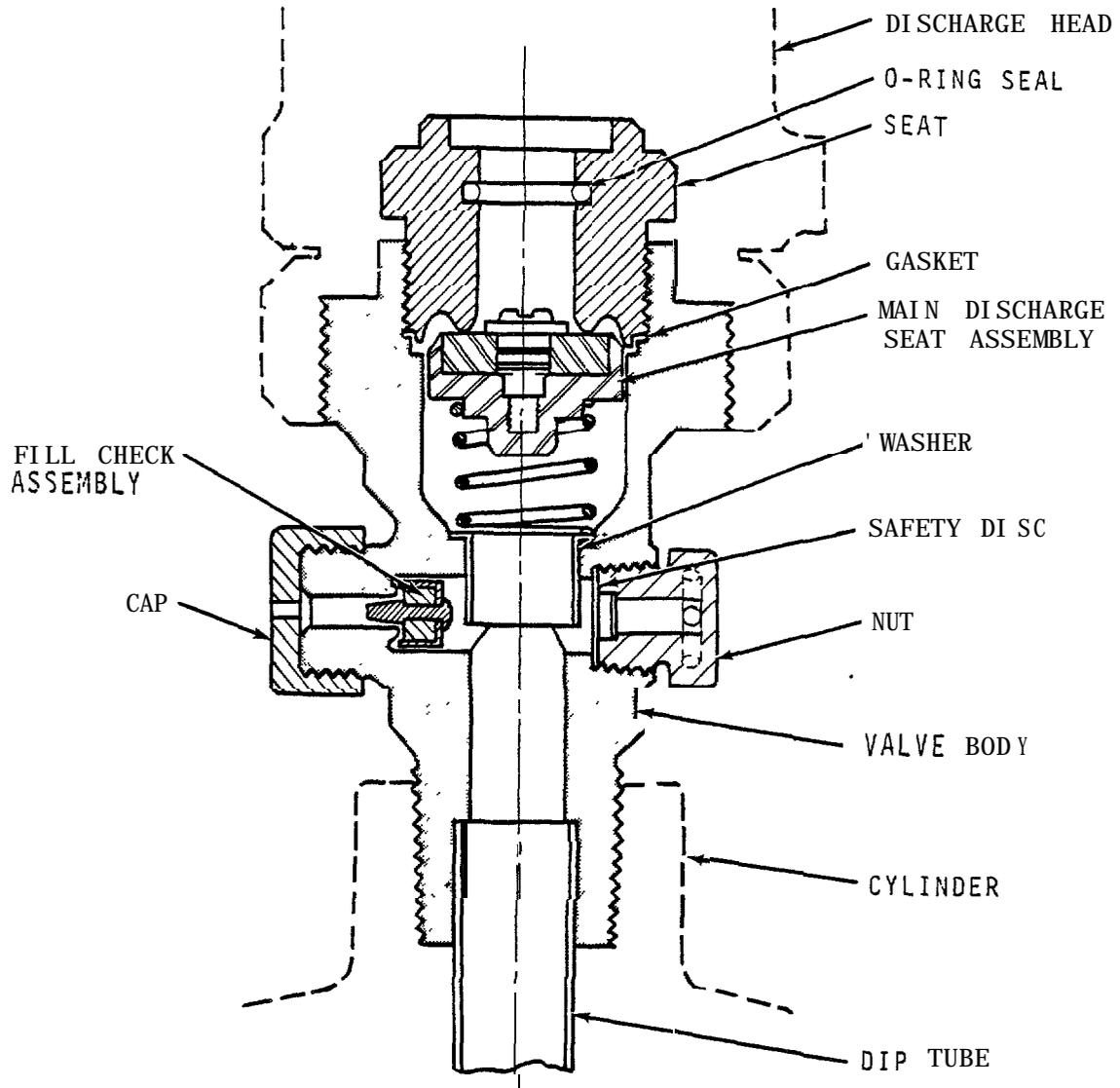
Figure 7. Cylinder Valve and Dip Tube.
