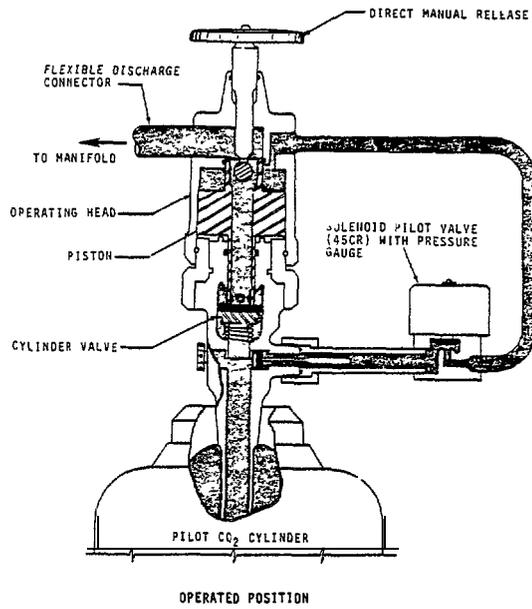
Figure 2. Pilot Cylinder Discharge Heads.
