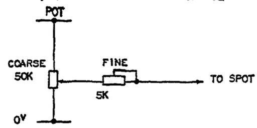
37 FIG. 1 - POTENTIOMETER ARRANGEMENT FOR VOLTAGE AND CURRENT SOURCE.
