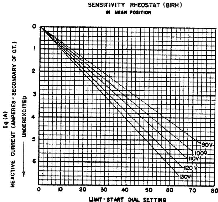
Figure 11. Calibration Curves For Reactive Ampere Limit Start Dial
