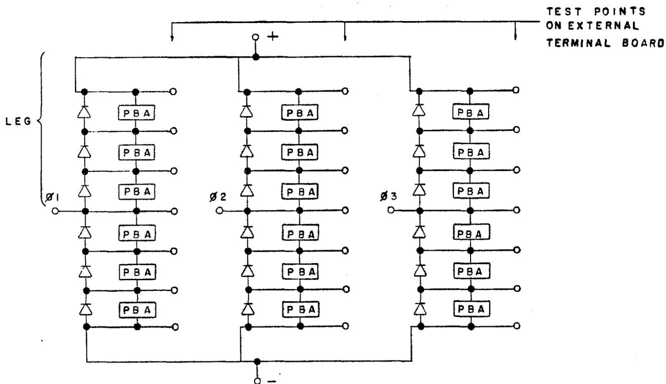
Figure 5. Electrical Connections of a Three-Phase Rectifier Bridge
