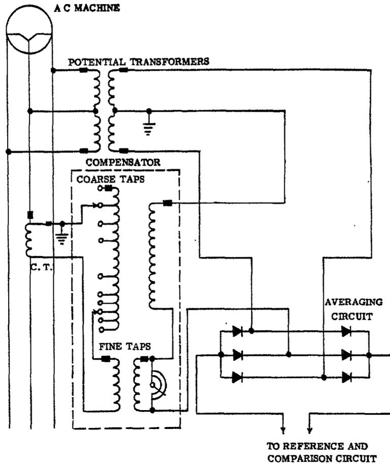
Figure 10. Active-and-Reactive Current Compensator Connections
