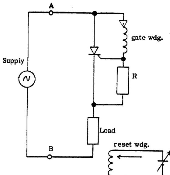
Figure 8. Simplified Version of SCR Circuit
