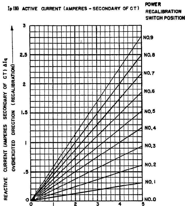
Figure 12. Calibration of Reactive-Ampere Power Recalibration Limit Circuit
