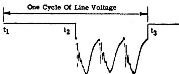
Figure 6. Wave-form Across One Diode When Operating Properly
