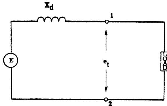
Figure 4. Simplified AC machine Equivalent Circuit
