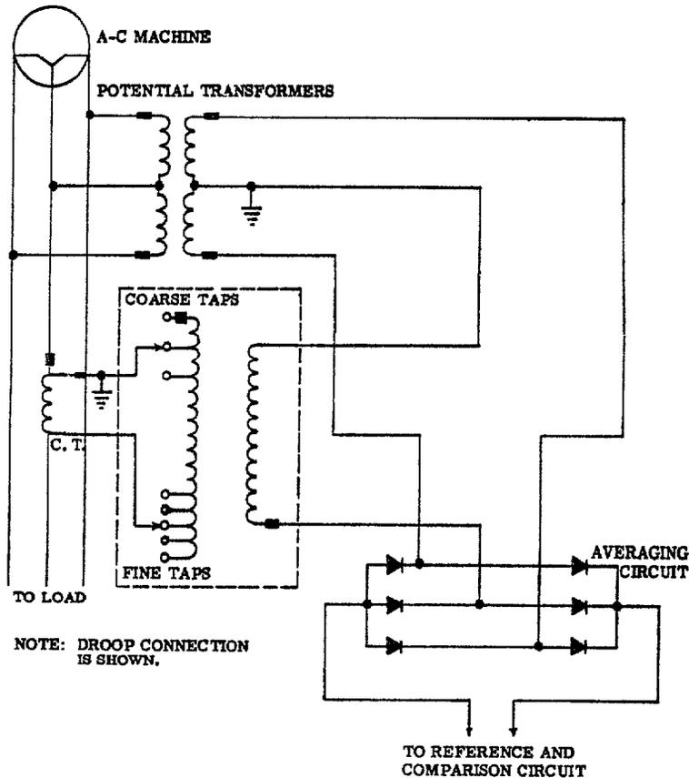
Figure 9. Reactive Current Compensator Connections
