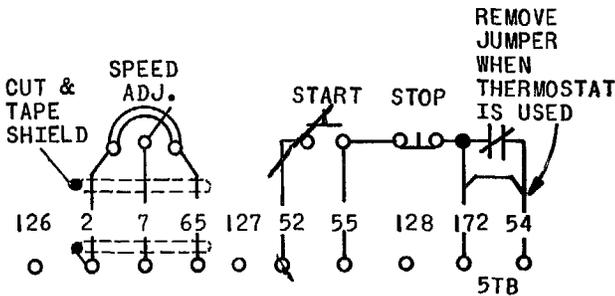
Figure 5. Remote Control Station Connection Diagram
