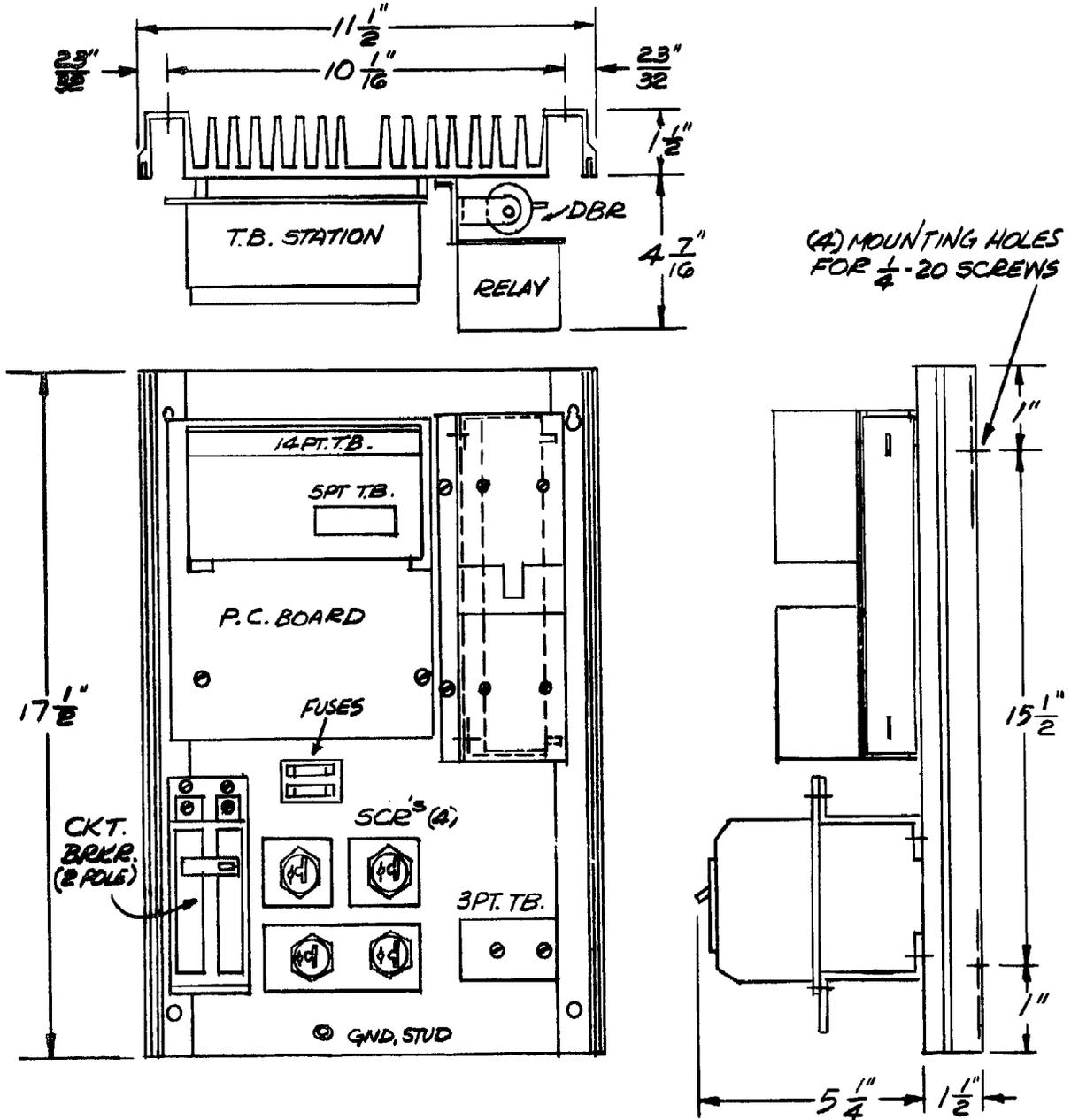
Figure 3. Outline and Mounting Dimensions for Chassis Mount Controller (3 and 5 HP) for use with Remote Control Station
