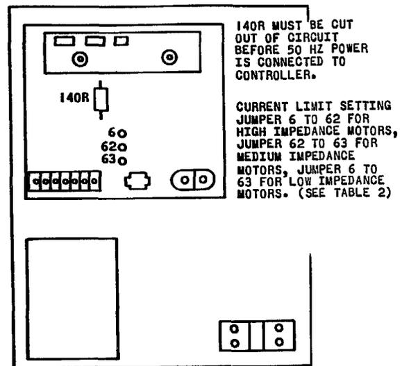
Figure 6. Current Limit Setting and 50 Hz Adjustment
