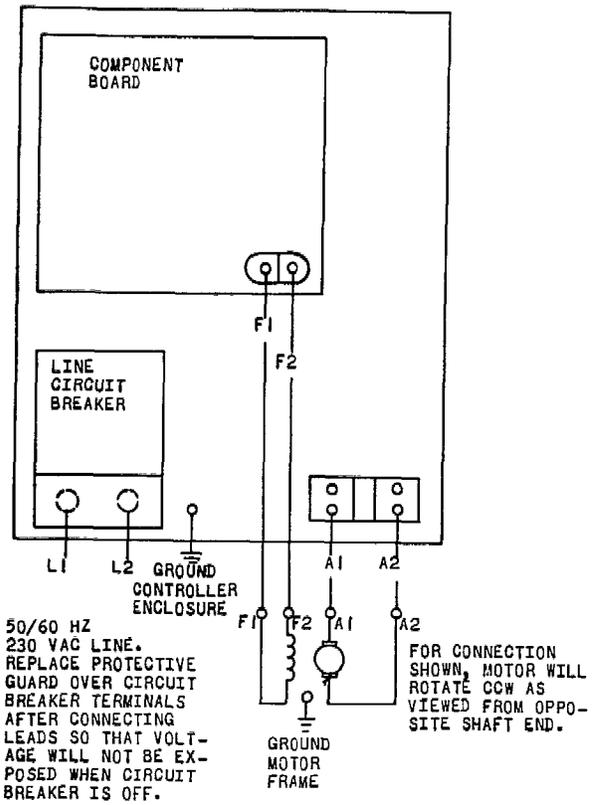
Figure 4. Power Wiring Connection Diagram
