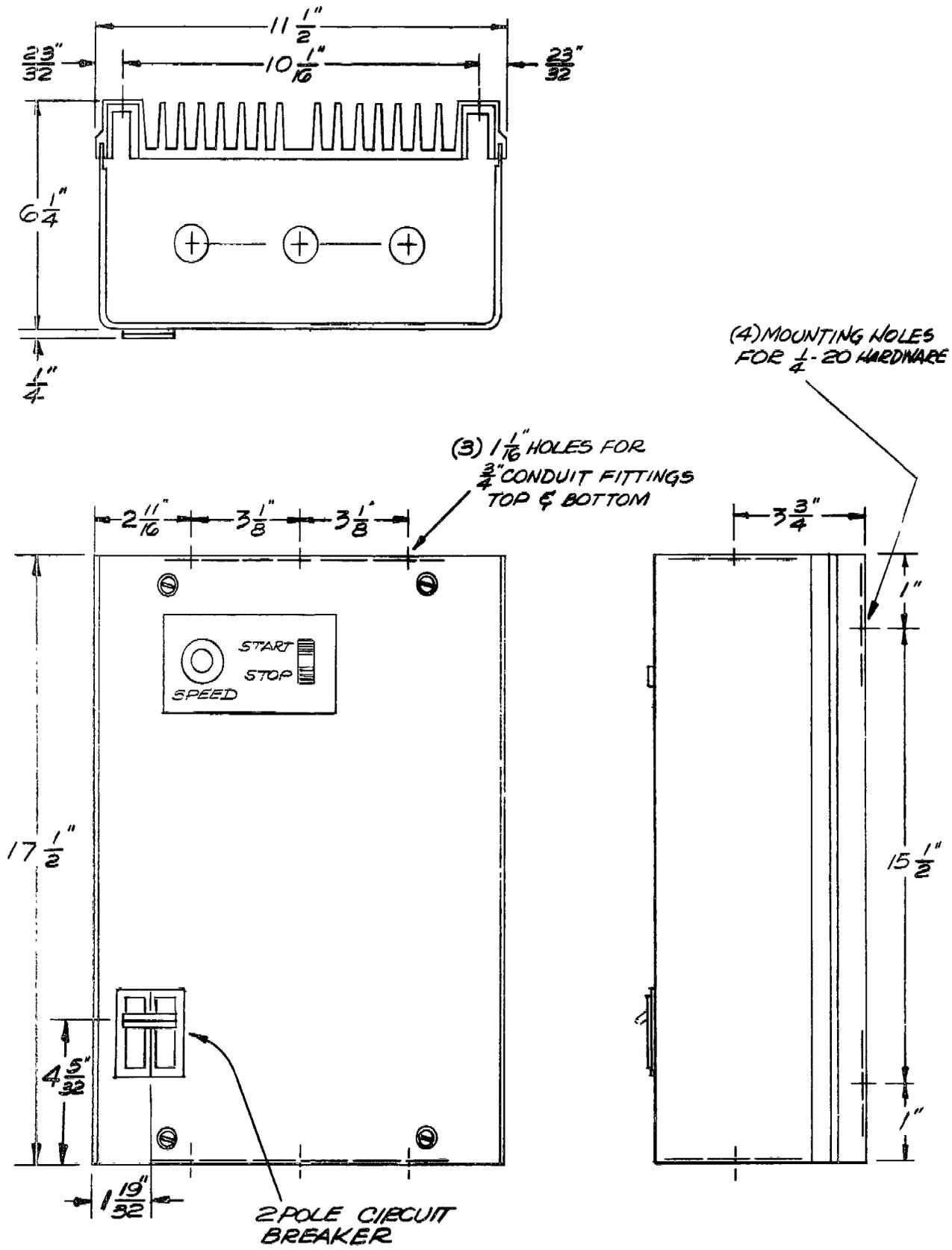
Figure 2. Outline and Mounting Dimensions for Enclosed Controller (3 and 5 HP) With Local Control Station
