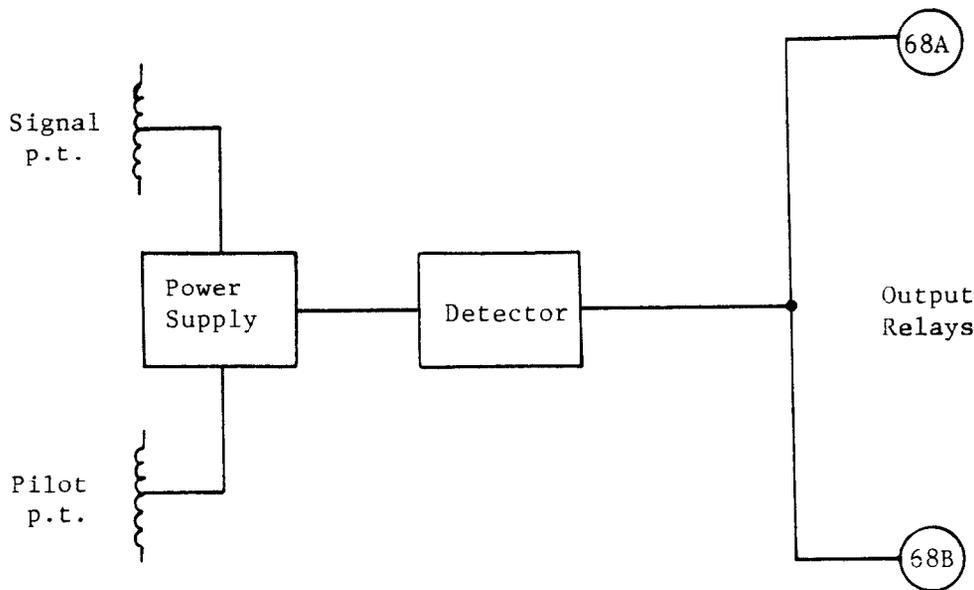
Figure 1. Voltage Balance Circuit
