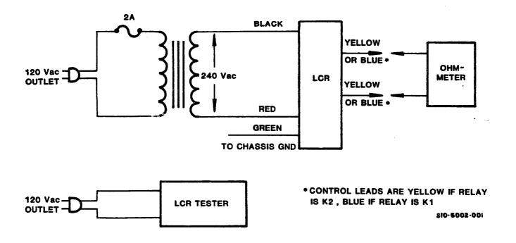
Figure 2-1. Bench Test Setup
