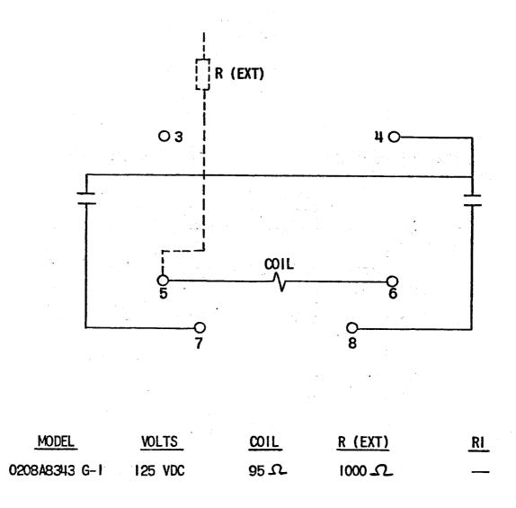
FIG. 1 (0246A2238-0) Internal Connections For Type HAA Model 208A8343
