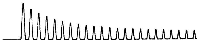
TYPICAL TRANSFORMER MAGNETIZING INRUSH CURRENT WAVE
