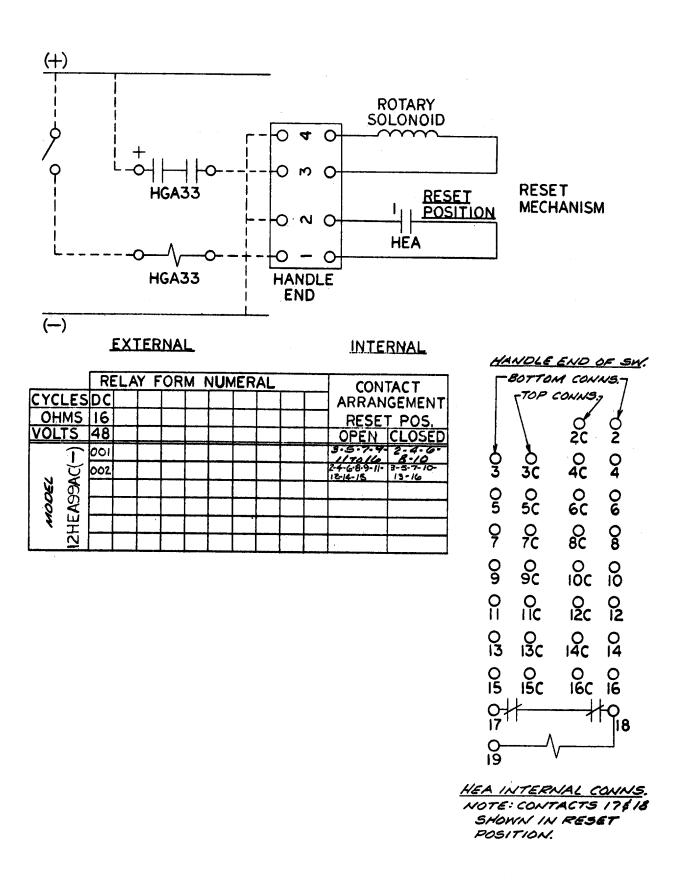
FIG. 1 (12HEA99AC-0 SH. 2) INTERNAL CONNECTIONS, OHMIC VALUE OF TRIP COIL, AND CONTACT ARRANGE-MENT FOR RELAY 12HEA99AC
