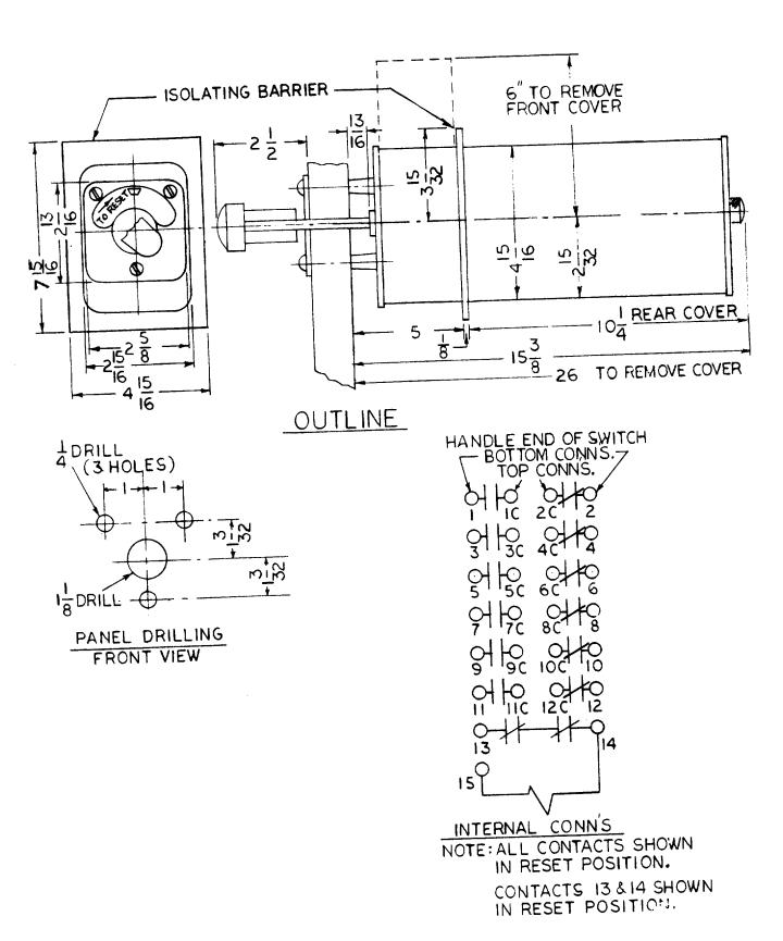
Fig. 1 (0269A1782-0) Internal Connections, Outline and Panel Drilling
