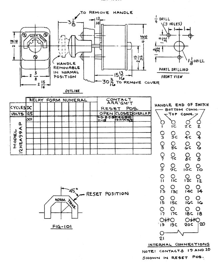
Fig. 1 (12HEA99AP-1 Sh. 2) Internal Connections, Outline and Panel Drilling for the 12HEA99AP Relay
