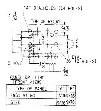
Figure 6 (0362A0576-6) Outline and Panel-Drilling Diagram for HFA154 Relays for Surface Mounting
