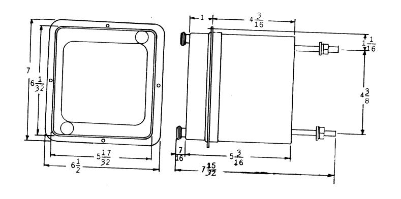
Figure 5 (637837-4) Outline and Panel-Drilling Diagram for HFA154 Relays for Semi-Flush Mounting
