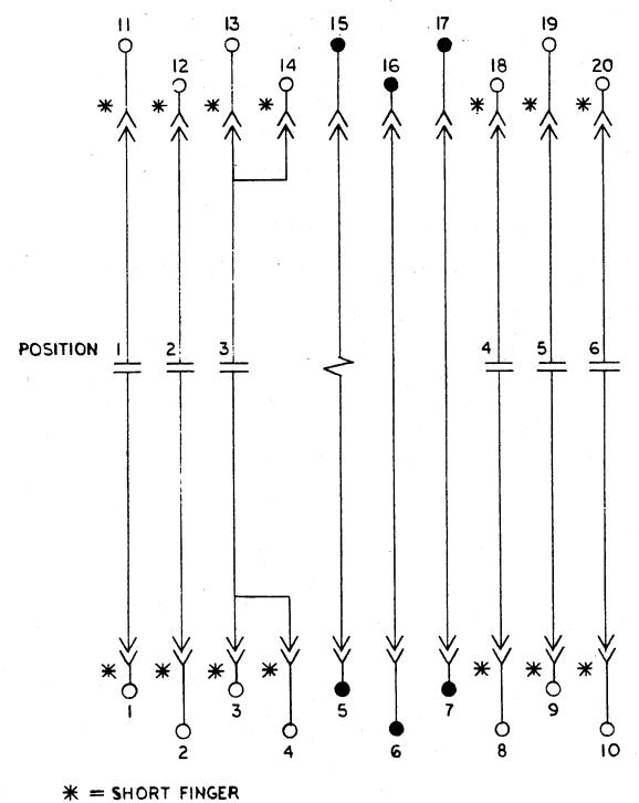
Fig.1 (0269A3054-0) Internal Connections Diagram for HFA99AG( )A Relay
