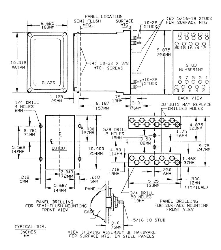
Figure 3 (K-6209272[7]) Outline and Panel-Drilling Diagram for HFA173K Relays
