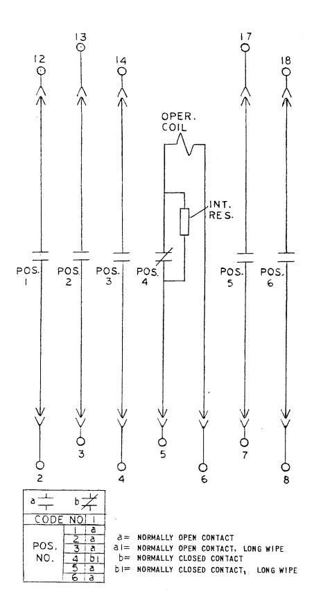
Figure 2 (0246A6960-0) Internal Connection Diagram for HFA173K Relays (Front View)
