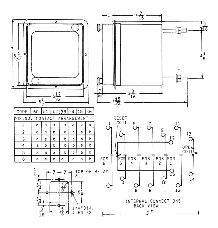
Figure 1 (K-6375837) Outline and Panel Drilling Dimensions, HFA99AP(-)F
