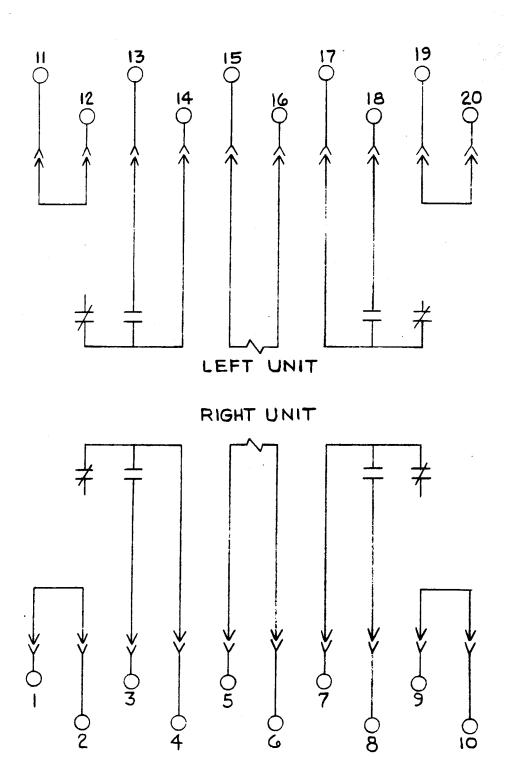
Fig. 1 (0208A2309-0) Internal Connections Diagram for the 12HGA99AF(-)A Relay
