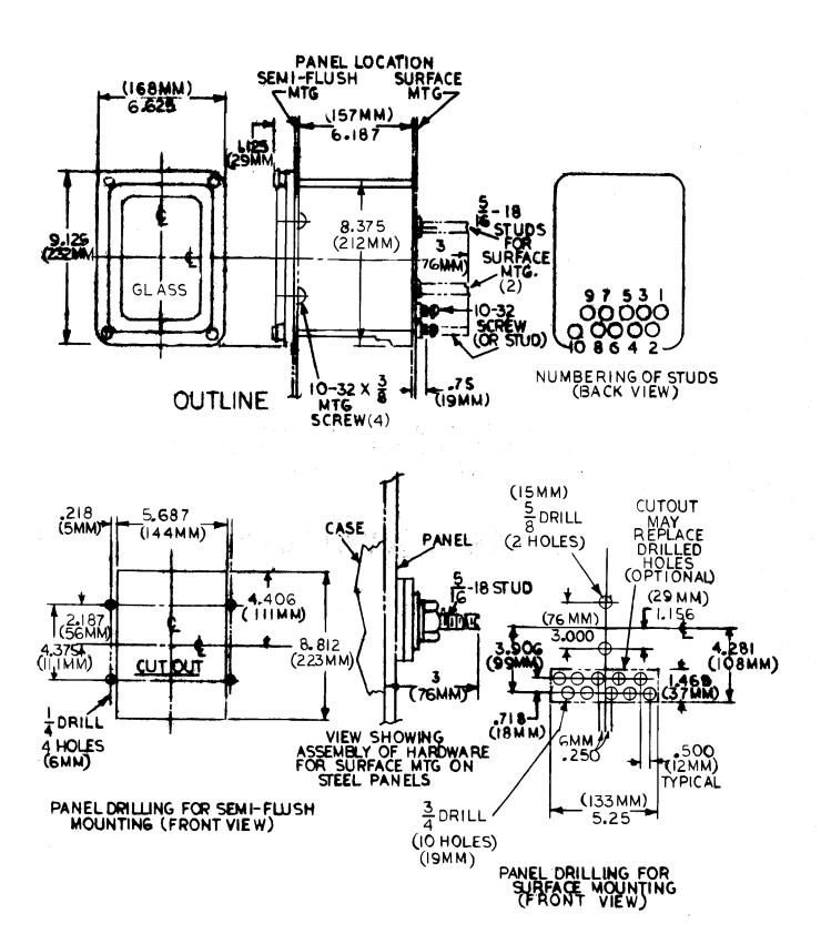
Fig. 5 (006209271-6) Outline and Panel Drilling Dimensions for the Type IAC99AS(-)A Relay
