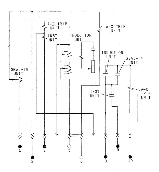
Fig. 3 (0376A0932-0) Internal Connections of the Type IAC99AS(-)A Relay (Front View)
