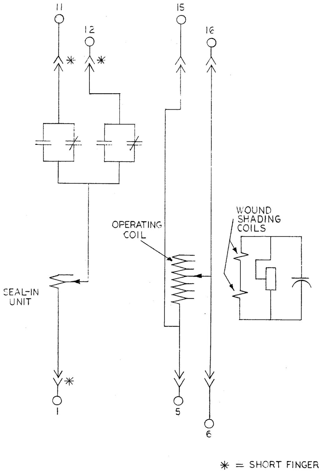
Fig. 1 (0275A2062-0) Internal Connection Diagram for 12IAV99AD
