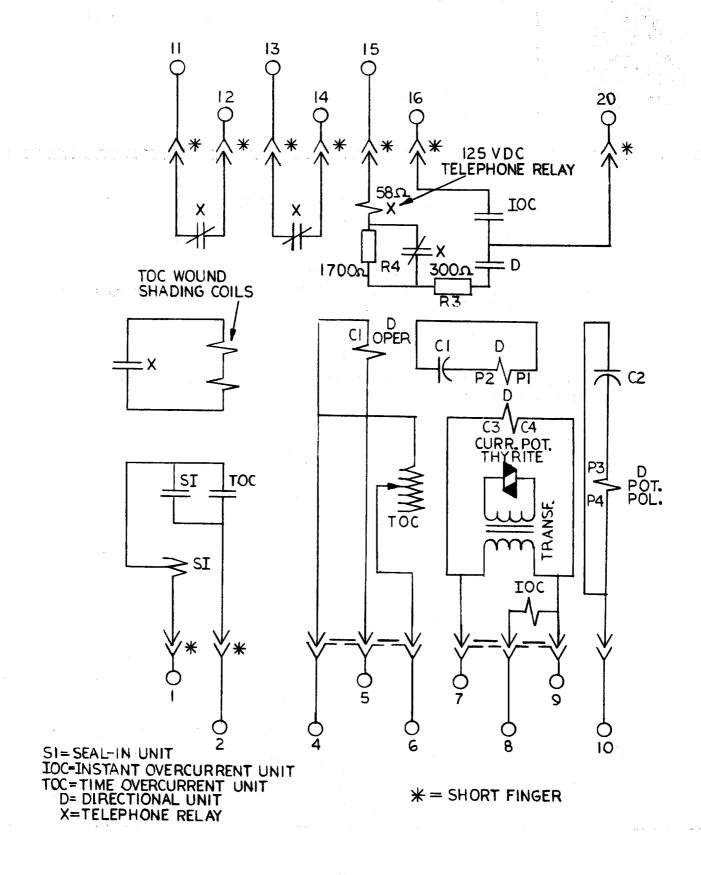
Fig. 1 (0275A2015-1) Internal Connections (Front View)
