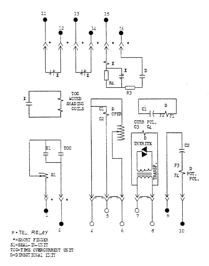
Figure 1 0178A9163-0 Internal Connections Diagram for the 0178A7374G(-) Relay
