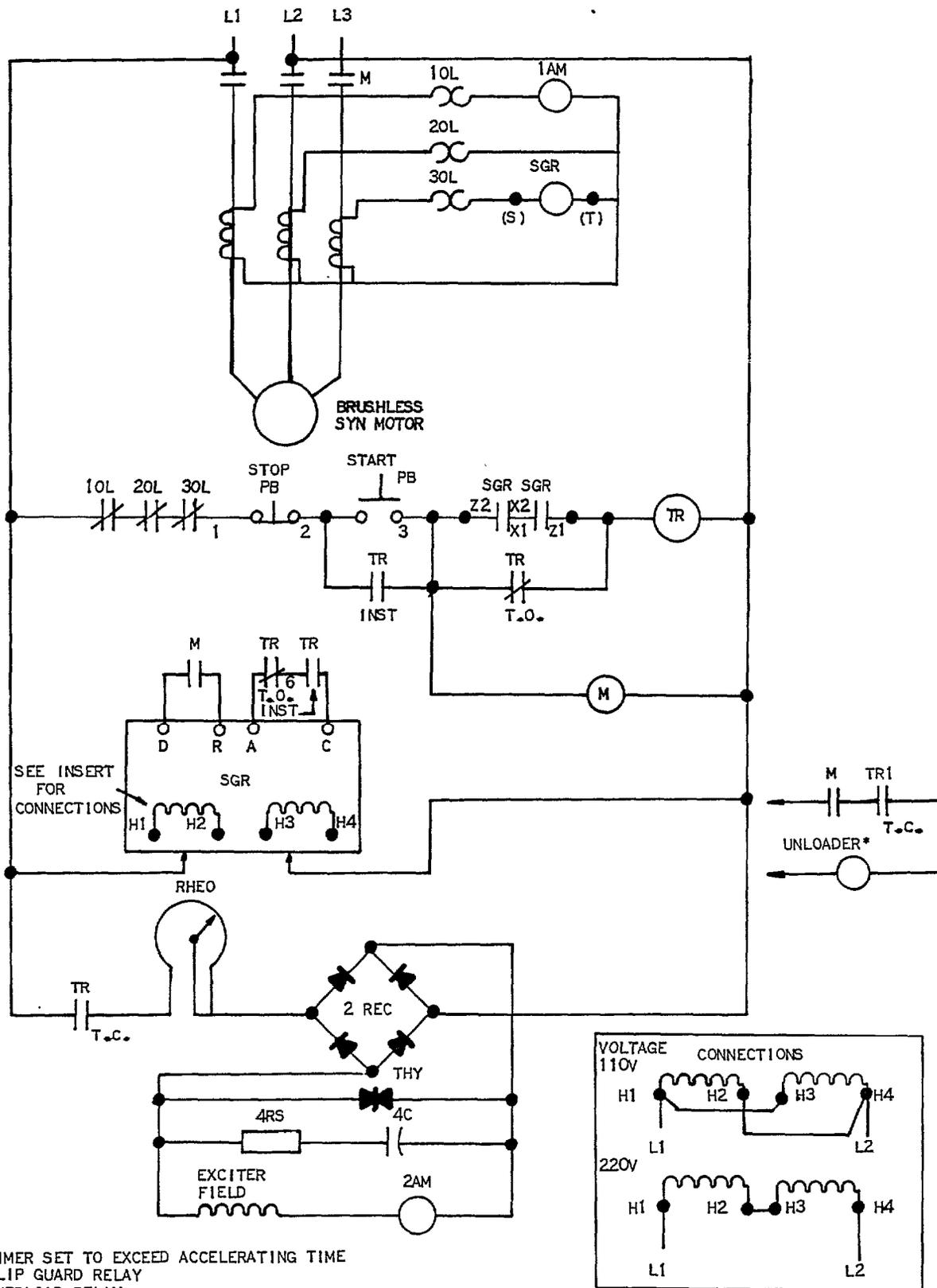
Typical Circuit for Brushless Synchronous Motor Control
