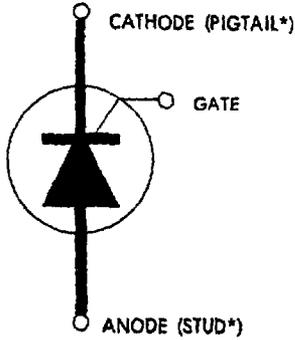
The SCR can be turned on by a momentary application of control current to the gate. To turn it off, it is necessary in addition to removing the turn-on signal from the gate, either to remove all power from the SCR or to apply momentary reverse voltage between cathode and anode.
