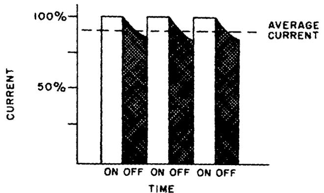
Fig. 6. Motor current
