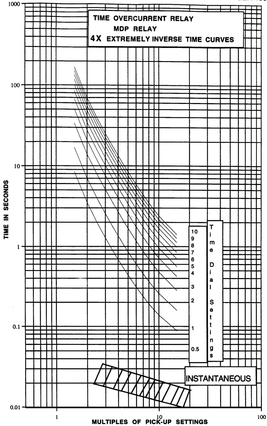
Figure 3 (0286A5627) MDP 4X Extremely Inverse Time Curve
