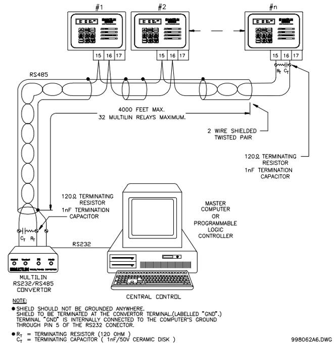
**Figure 2.1** Serial Communication Link
