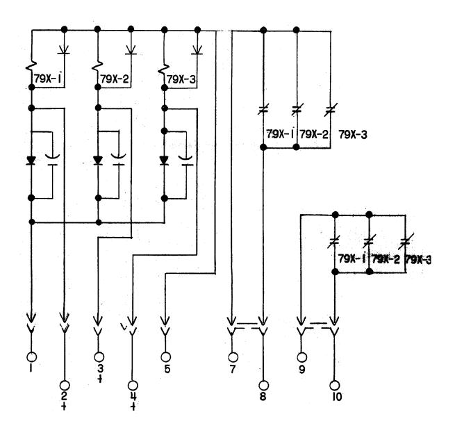
Fig. 1 (0257A5081-0) INTERNAL CONNECTION DIAGRAM FOR SPECIAL RELAY 12NAA99AC001A RELAY
