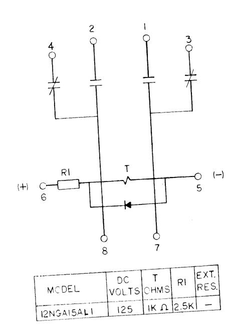
Figure 1 (0286A2814) Internal Connections Diagram for 12NGA15AL(-) Relay 5/90-200 GENERAL ELECTRIC METER AND CONTROL BUSINESS DEPT., MALVERN, PA 19355
