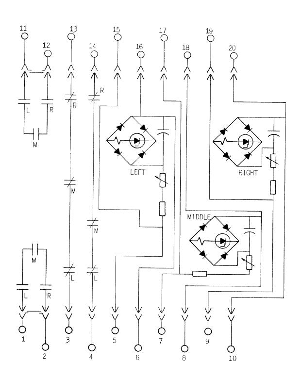
FIG. 1 (0226A6930-0) Internal Connections Diagram For The NGV11D Relay
