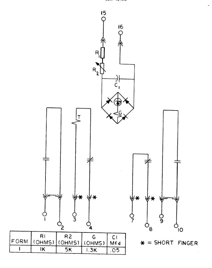
FIG. 1 (269A3034- 0 ) INTERNAL CONNECTIONS DIAGRAM FOR THE NGV28B(-)A RELAY.
