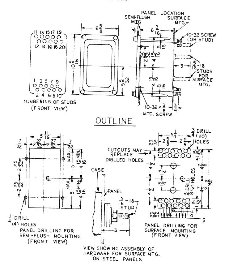
FIG. 2 (K-6209272) OUTLINE AND PANEL DRILLING DIMENSIONS FOR THE NGV28B(-)A RELAY-SIZE S2 CASE.
