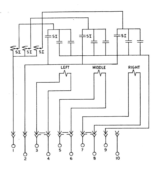
Figure 1 (0273A9541-0) Internal Connections Diagram for the 12PJC99AF(-)A Relay
