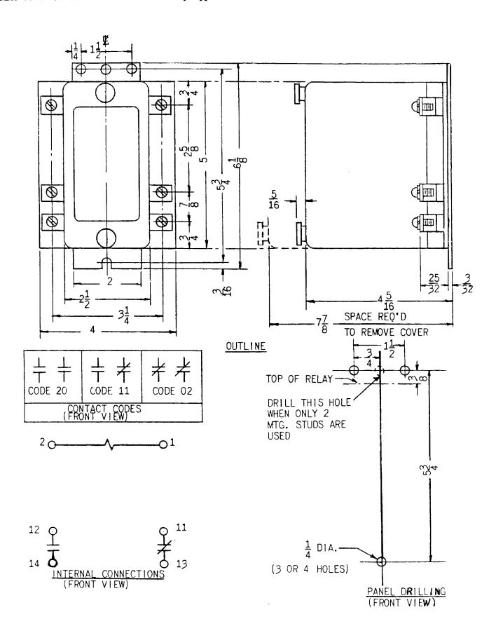
Fig. 1 (0165A7526-1) Outline And Panel Drilling Dimensions For Pelsy Type BJC11BA.
