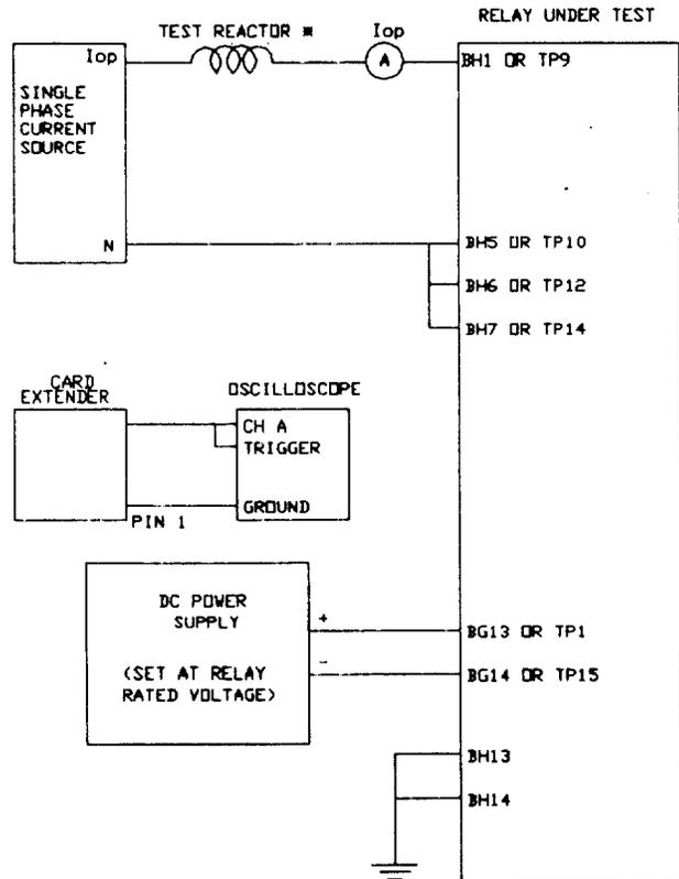
Figure AT-6 (0285A9843 [1]) IT Test Connections
