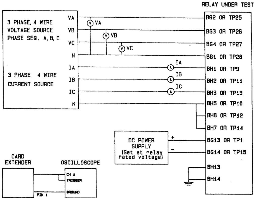
Figure AT-3 (0285A9840 [1]) Positive-Sequence Distance Test Connections
