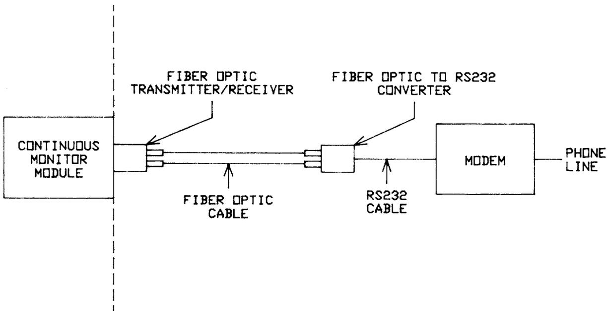
Figure CM-2 (0285A9899 [2]) Serial Data Link Connection
