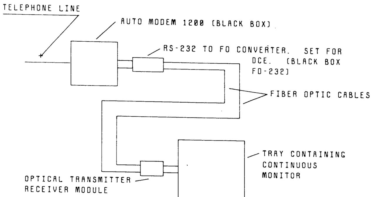
Figure CM-3 (0285A9836 [1]) Continuous Monitor Phone Connection
