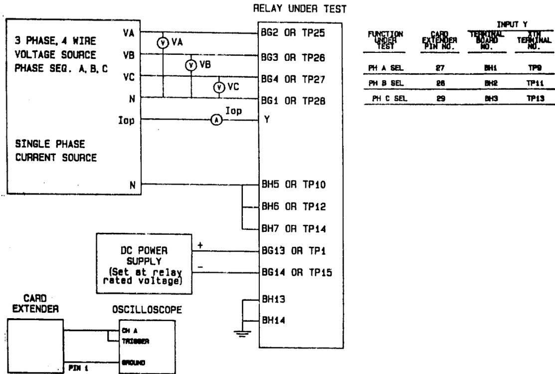
Figure AT-5 (0285A9842 [1]) Negative-Sequence Directional Test Connections and Phase Selectors Test Connections
