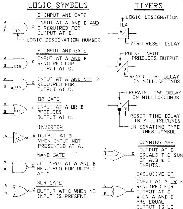
Figure SD-2 (0286A2775 Sh.1 [3]) Logic and Internal Diagram Legend
