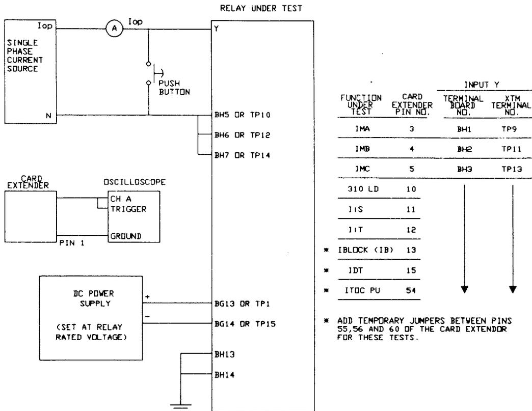
Figure AT-1 (0285A9838 [1]) Level Detector Test Connections
