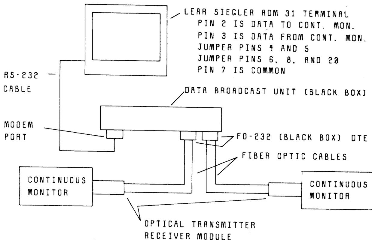
Figure CM-4 (0285A9837 [1]) Connection for Multiple Continuous Monitors
