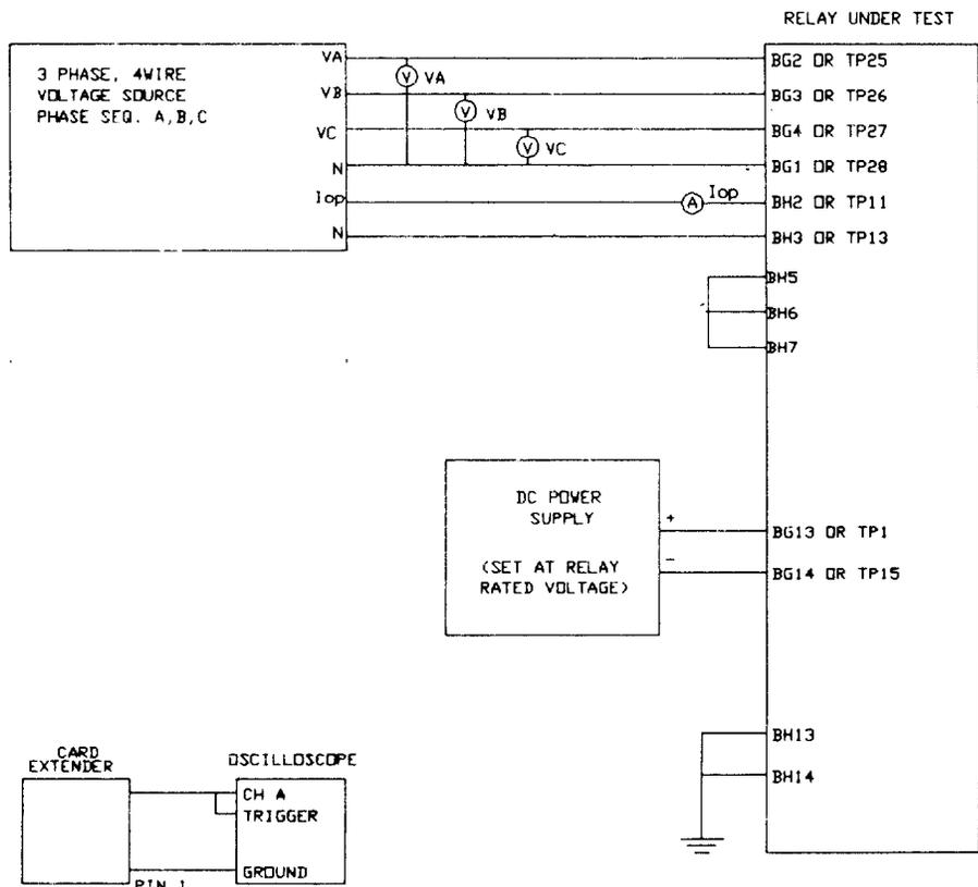
Figure AT-4 (0285A9841 [2]) Negative-Sequence Distance Test Connections
