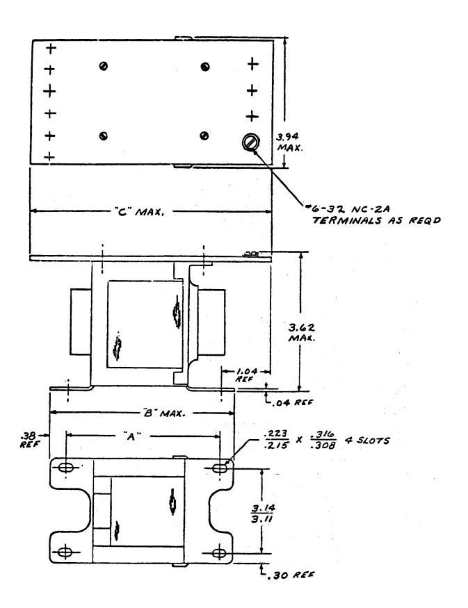
Fig. 2 (467A716AA-7) Outline of Test Transformer (9T58B2909)
