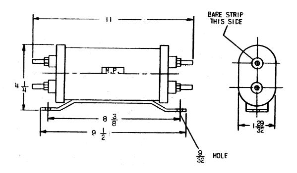
Fig. 4 (403A119-1) Outline of Test Resistor
