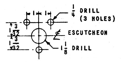
Fig. 5 (0116A0130-7) Panel Drilling Dimensions Diagram for Test Switch (Type SB-1 Switch)
