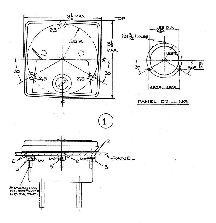
Fig. 6 (381A128-0) Outline and Panel Drilling for Semi-flush Mounted Meter (Type DO-91)
