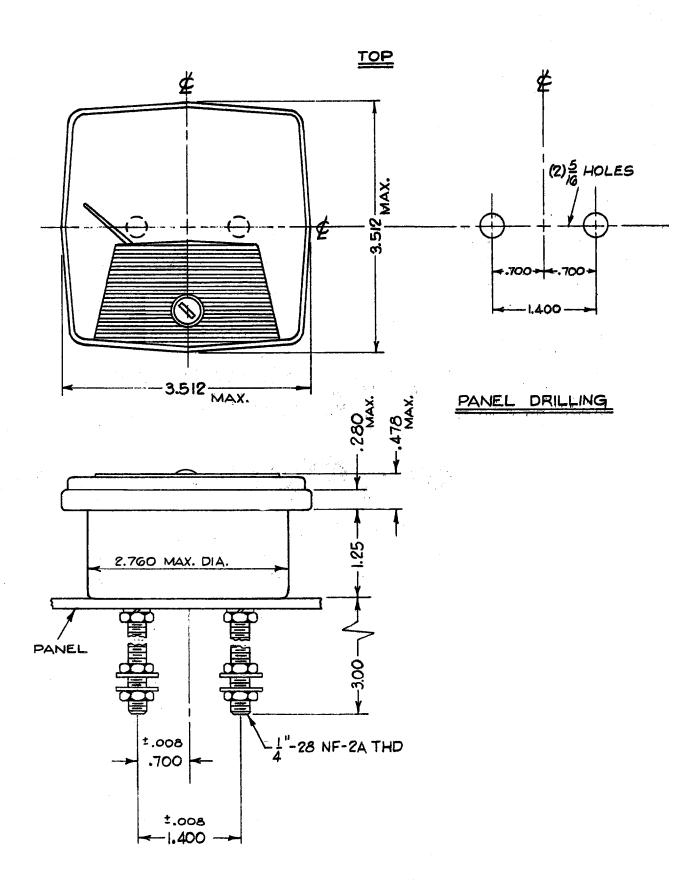
Fig. 7 (0148A3872-0) Outline and Panel Drilling for Surface Mounted Meter (Type D0-91)
